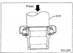
Install release bearing with suitable drift.
