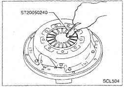
Adjust unevenness of diaphragm spring with Tool.
