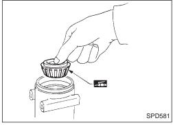
4. Place pinion front bearing inner cone in gear carrier.
