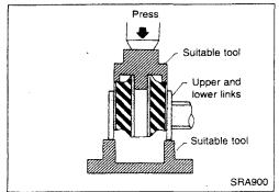
When installing bushing, apply a coating of 1% soap water to outer wall of bushing.
