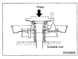
Install baffle plate over bearing housing and press axle shaft into inner race of wheel bearing.
