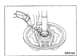
Secure lock nut by bending one portion of lock washer.
