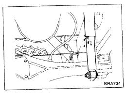
Check shock absorber for oil leakage or other damage.
