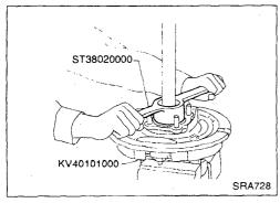
Remove bearing lock nut with Tool.
