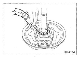
Unbend lock washer with a screwdriver.
