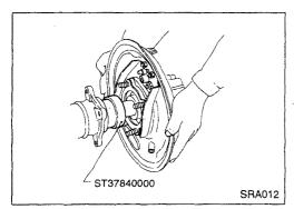
Insert axle shaft with Tool as a guide.
