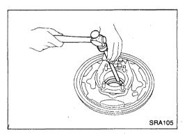
Remove grease seal in bearing cage with suitable bar.
