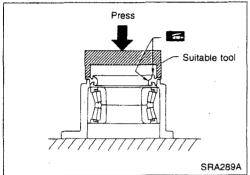
Press new grease seal until it bottoms end face of bearing housing.
