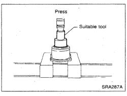
Remove wheel bearing outer race with a suitable tool.
