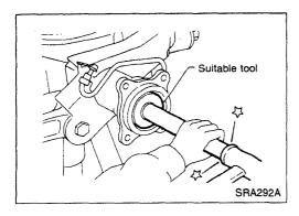
Install new oil seal to rear axle housing using a suitable tool.
