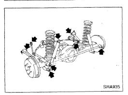
Final tightening for rubber parts requires to be carried out under unladen condition with tires on ground.
