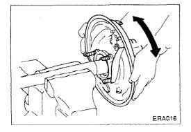
Turn bearing housing (with respect to axle shaft) two or three times. It must turn smoothly.
