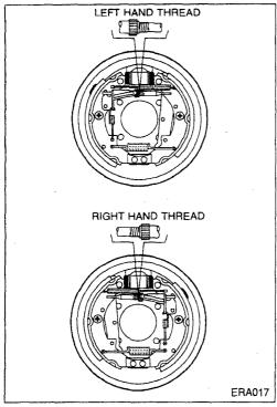
When the ball-bearing holder and the brake are installed in the base of the axle, they need to be correctly positioned.
