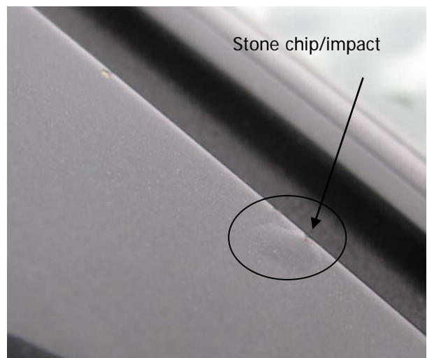
Example of non-warranty paint blister: cause - stone chipping
