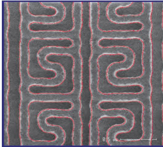
**Figure 7.105** Model-generated edge contour superimposed on the resist image (image courtesy of R.G. Liu).
