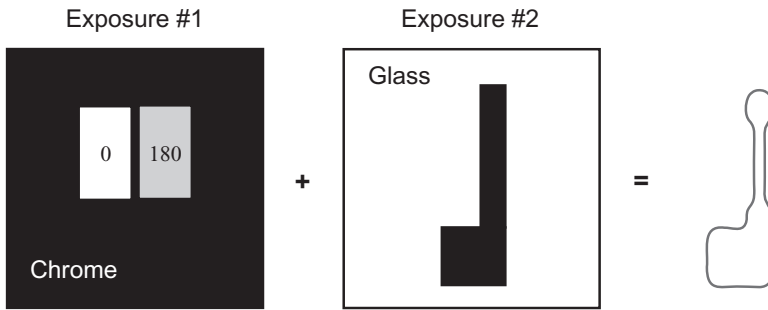
Figure 10.28 Simple example of a double-exposure alternating phase-shift mask approach to gate-level patterning
