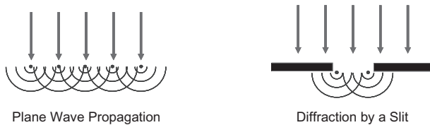
Figure 2.2 Pictorial representation of Huygens' principle, where any wavefront can be thought of as a collection of point sources radiating spherical waves
