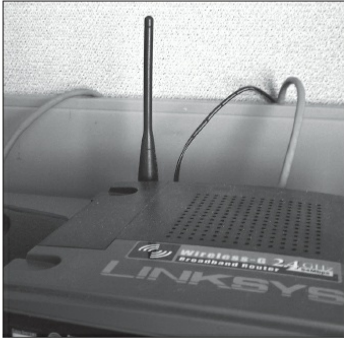
Figure 1.11 — Typical 2.4 GHz monopole antenna, functionally nearly identical to the AM broadcast antenna. The only significant difference is operation frequency and thus size! As operating frequencies have increased over time, some of the simplest antenna types were simply made smaller and smaller and smaller.
