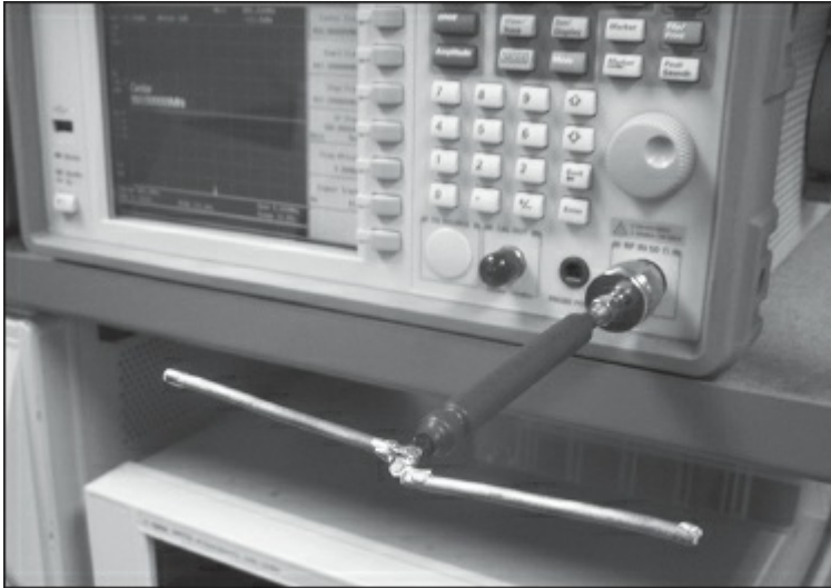
Figure 2.15 — A simple dipole antenna for 950 MHz. [Courtesy of Trimble Navigation Ltd]
