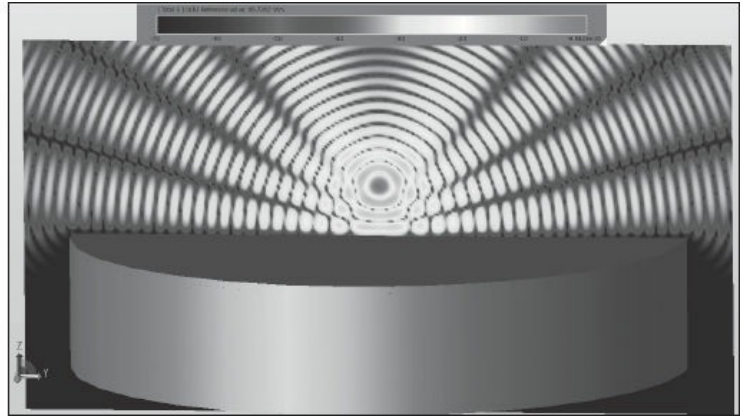
Figure 6.6 — This figure shows an EMPro simulation of a horizontal \frac{1}{2}\lambda dipole at 2\lambda height over real ground. The view is down the axis of the dipole, thus highlighting the broadside E -field pattern of the dipole. This view also shows a disc representing the real “average” ground. This type of electromagnetic simulation permits a view of the nulling and reinforcing of waves at different take-off angles.
