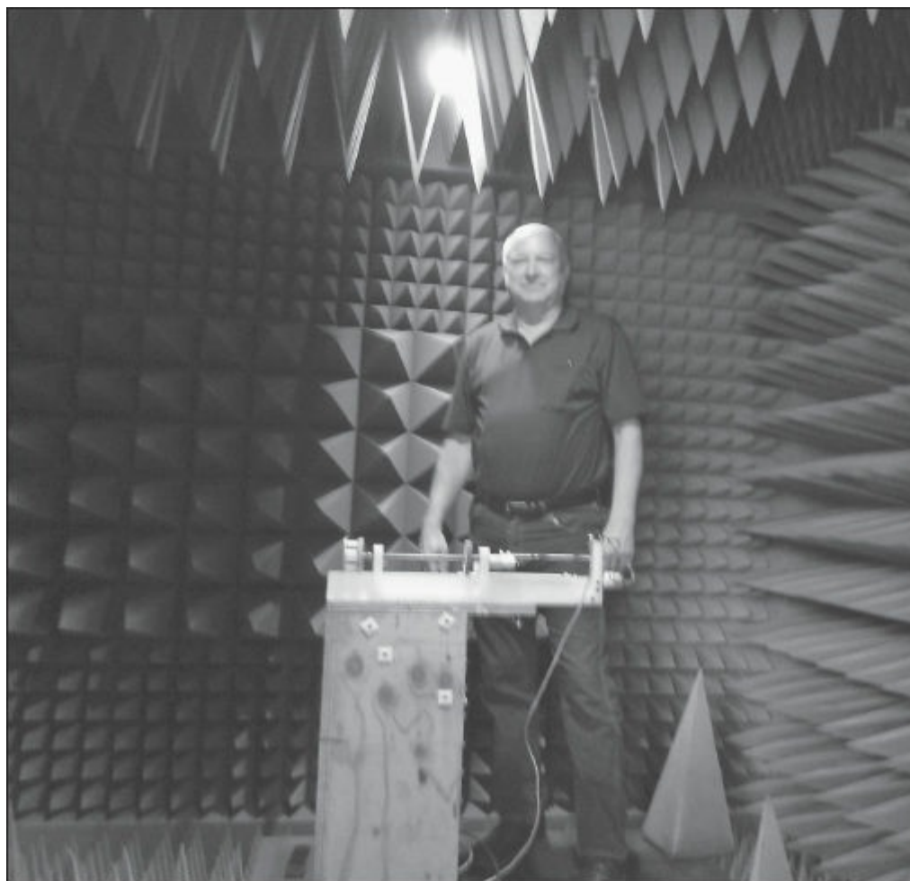
Figure 2.5 — The author inside an anechoic chamber used to simulate free space antenna testing. [Courtesy of Trimble Navigation Ltd]
