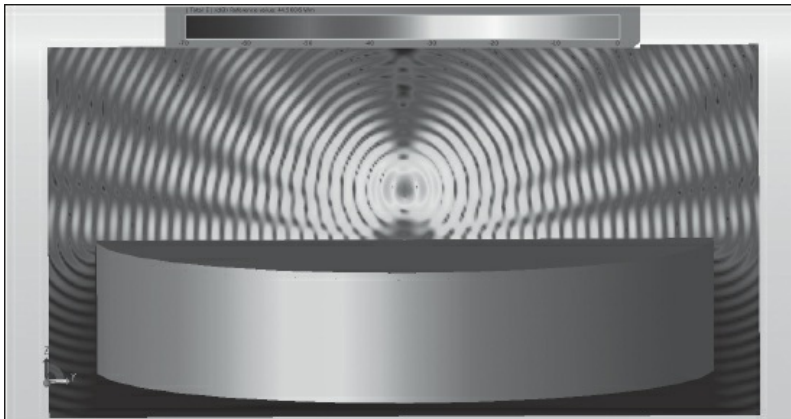
Figure 6.11 — This is a plot of an elevated \frac{1}{2} \lambda vertical dipole (two wavelengths high) over a large slab of average ground. In this case we can clearly see the effects of reflected waves, with interfering and reinforcing fields creating the final pattern.
