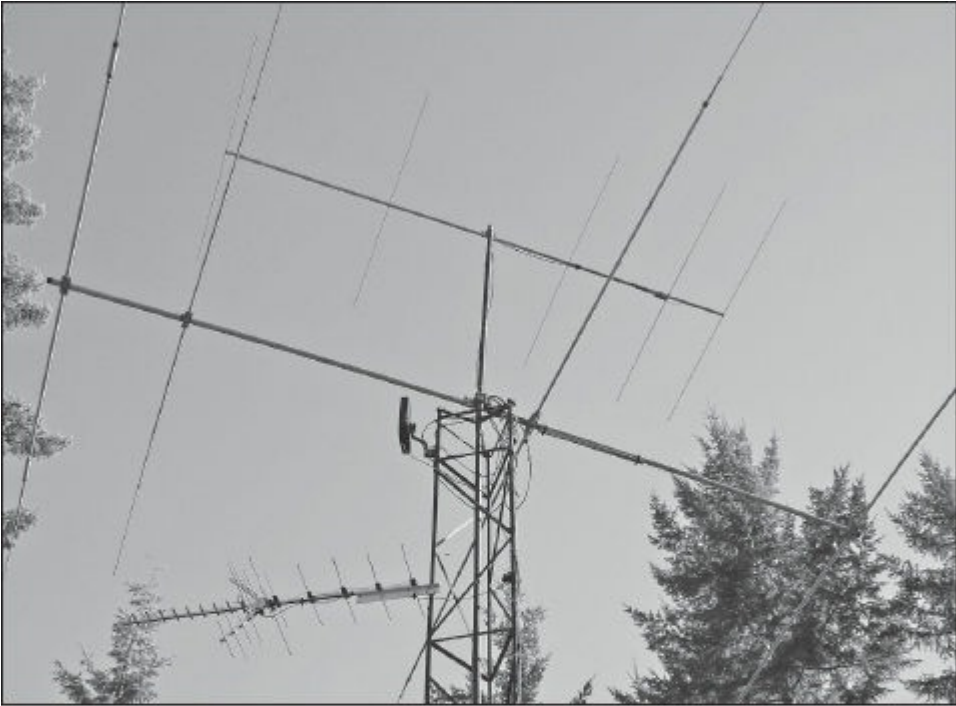
Figure 2.3 — The author's home-built tower: Amateur Radio operators are frequent users of the reciprocity theorem for two-way communications around the world. Featured in this photo are three Yagi-Uda arrays, which is really a direct spin-off of the simple dipole. Notice the shorter dipole lengths on the top antenna for the VHF being covered (50 MHz) vs. the Yagi below for the 14 and 21 MHz HF bands. The antennas are used for both transmitting and receiving. Also shown is a UHF TV broadcast antenna. [Photo by the author. Tower design, fabrication, and welding also by the author.]
