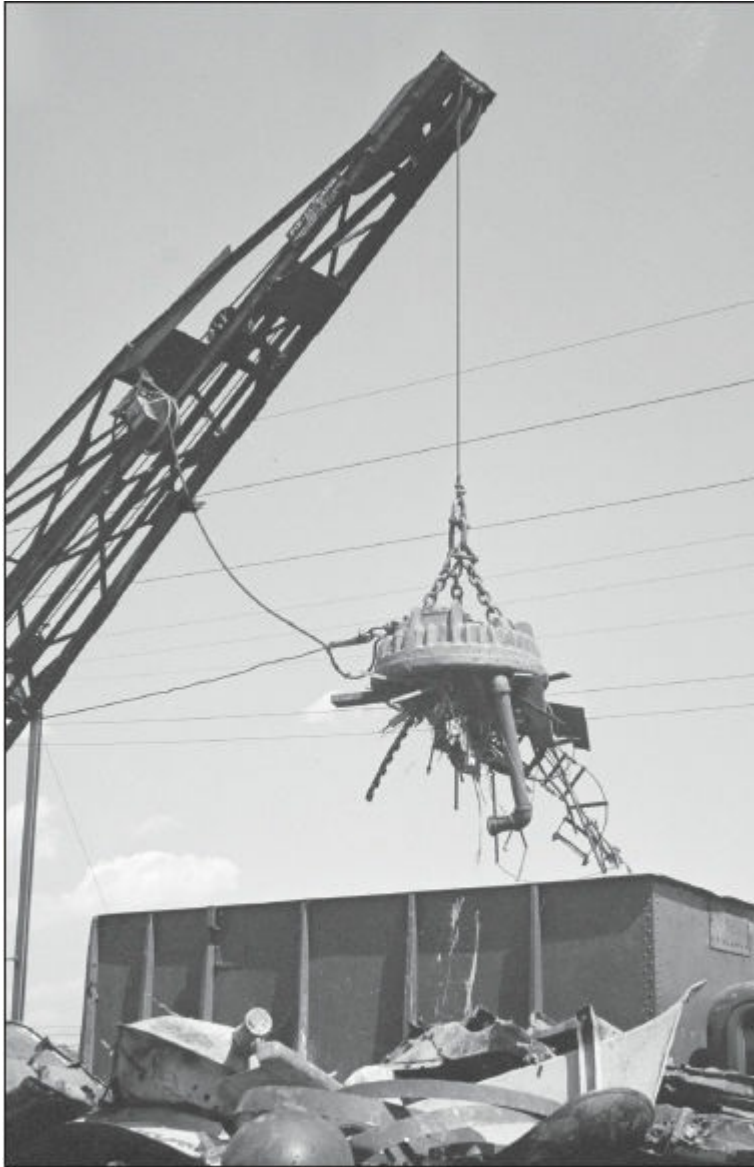
Figure 3.5 — Ampere's Law at work in this giant electromagnet: a moving charge (current) flowing in a loop creates a magnet. Turn the current off and the magnetic field disappears. [Library of Congress, Prints & Photographs Division, FSA/OWI Collection, LC-DIG-fsa-8c34729]
