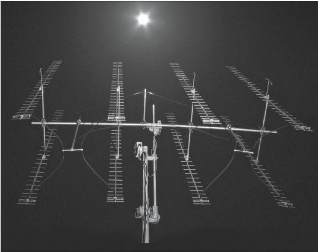
Figure 8.11 — This array of eight long Yagi-Uda antennas is intended for 432 MHz “moonbounce” or EME (Earth-Moon-Earth) amateur communications. Each antenna has 27 elements. If each Yagi-Uda has a 20 dBi gain, then the theoretical possible gain from eight antennas is 29 dBi. [Noriyuki Yaguchi, JH0WJF, photo]
