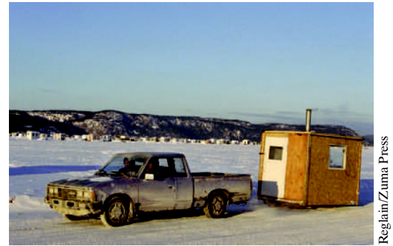
Figure 7.6.1 The power due to the truck's applied force on the trailing load is the rate at which that force does work on the load.
