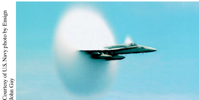
Figure 17.8.2 Shock waves produced by the wings of a Navy FA 18 jet. The shock waves are visible because the sudden decrease in air pressure in them caused water molecules in the air to condense, forming a fog.
