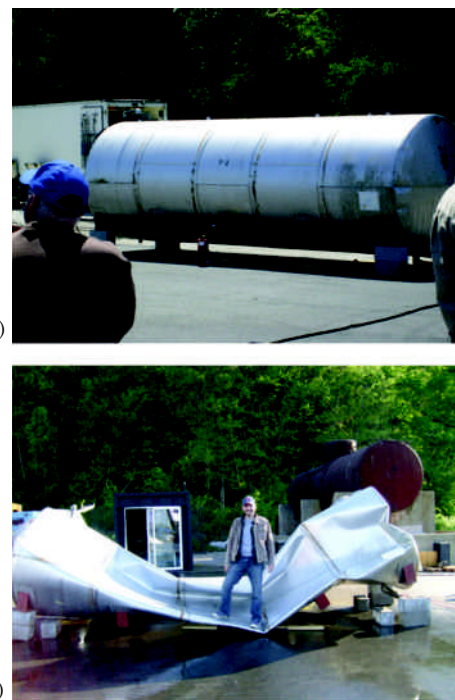
Figure 19.2.1 (a) Before and (b) after images of a large steel tank crushed by atmospheric pressure after internal steam cooled and condensed.
