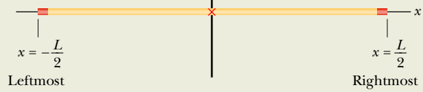
Figure 10.5.3 A uniform rod of length L and mass M . An element of mass dm and length dx is represented.
