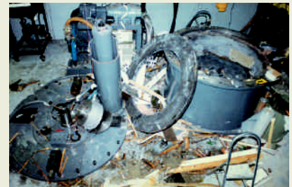
Figure 10.5.4 Some of the destruction caused by the explosion of a rapidly rotating steel disk.
