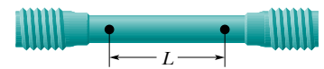
Figure 12.3.4 A test specimen used to determine a stress–strain curve such as that of Fig. 12.3.5. The change \Delta L that occurs in a certain length L is measured in a tensile stress–strain test.
