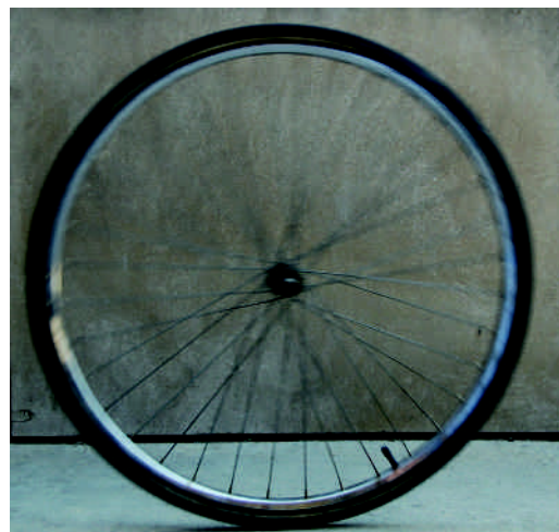
Figure 11.1.5 A photograph of a rolling bicycle wheel. The spokes near the wheel's top are more blurred than those near the bottom because the top ones are moving faster, as Fig. 11.1.4c shows.
