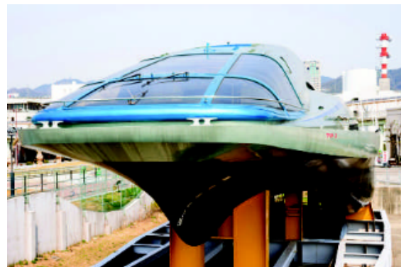
Figure 28.3.3 The Yamato-1 was a full-scale ship driven by the magnetohydrodynamic effect.
