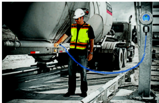
Figure 27.67 Problem 101. A grounding cable runs from truck into post and then down into the ground.
