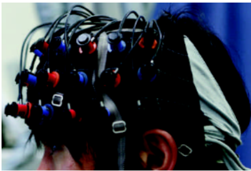
Figure 34.5.4 In functional near infrared spectroscopy (fNIRS), a person wears a close-fitting cap with LEDs emitting in the near infrared range. The light can penetrate into the outer layer of the brain and reveal when that portion is activated by a given activity, from playing baseball to flying an airplane.
