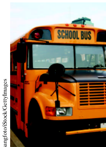
Figure 34.2.2 A crossover mirror allows a truck or bus driver to see a pedestrian in the blind spot in front of the vehicle.
