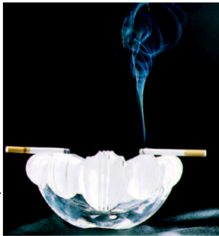
Figure 14.6.1 At a certain point, the rising flow of smoke and heated gas changes from steady to turbulent.
