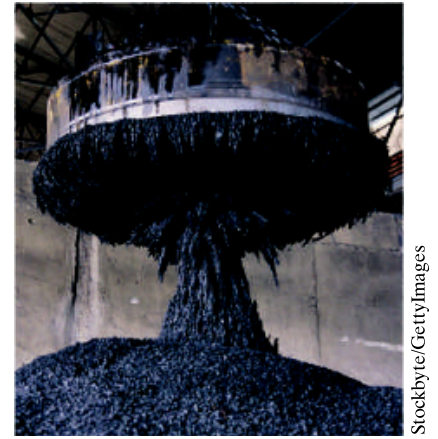
Figure 28.1.1 Using an electromagnet to collect and transport scrap metal at a steel mill.
