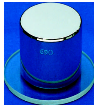
Figure 1.3.1 The international 1 kg standard of mass, a platinum–iridium cylinder 3.9 cm in height and in diameter.
