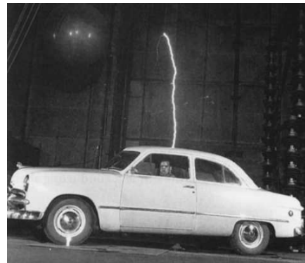
Figure 24.8.2 A large spark jumps to a car's body and then exits by moving across the insulating left front tire (note the flash there), leaving the person inside unharmed.
