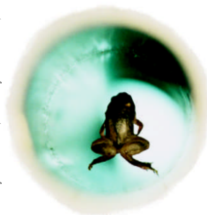
Figure 32.6.1 An overhead view of a frog that is being levitated in a magnetic field produced by current in a vertical solenoid below the frog.
