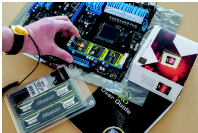
Figure 27.55 Problem 75. Wrist strap to discharge static electric charge.
