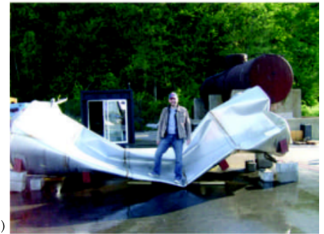
Figure 19.2.1 (a) Before and (b) after images of a large steel tank crushed by atmospheric pressure after internal steam cooled and condensed.
