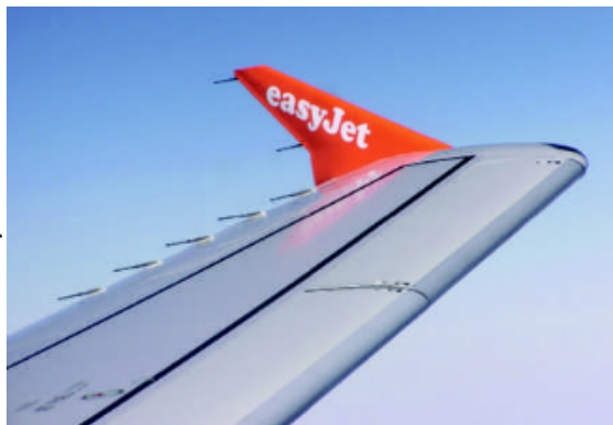
Figure 24.8.3 The static wicks continuously discharge to the air to avoid the airplane becoming highly charged with the possibility of a large and disastrous discharge spark.
