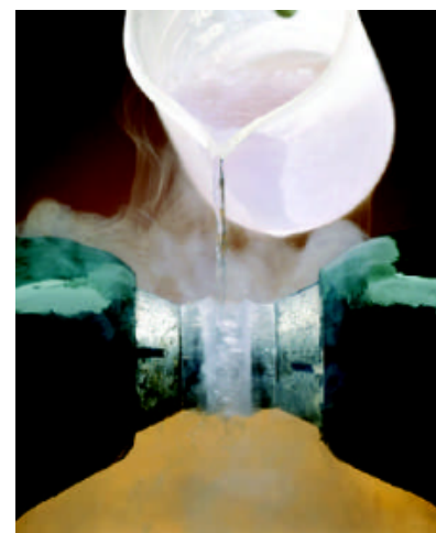
Liquid oxygen is suspended between the two pole faces of a magnet because the liquid is paramagnetic and is magnetically attracted to the magnet.
