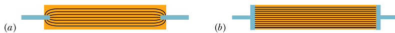
Figure 26.3.2 Two ways of applying a potential difference to a conducting rod. The gray connectors are assumed to have negligible resistance. When they are arranged as in (a) in a small region at each rod end, the measured resistance is larger than when they are arranged as in (b) to cover the entire rod end.
