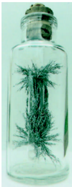
Figure 28.1.4 (a) The magnetic field lines for a bar magnet. (b) A “cow magnet”—a bar magnet that is intended to be slipped down into the rumen of a cow to prevent accidentally ingested bits of scrap iron from reaching the cow’s intestines. The iron filings at its ends reveal the magnetic field lines.
