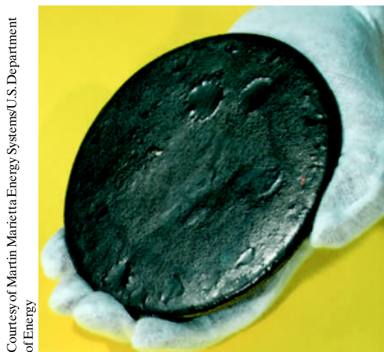
Figure 43.1 Problem 15. A “button” of ^{235}\text{U} ready to be recast and machined for a warhead.
