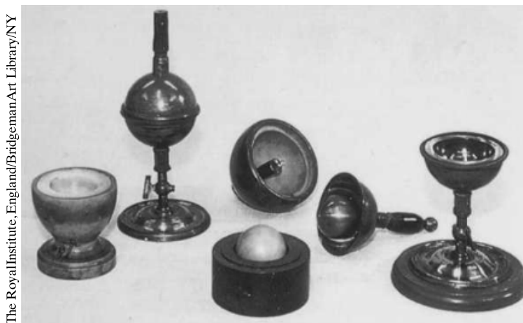
Figure 25.5.1 The simple electrostatic apparatus used by Faraday. An assembled apparatus (second from left) forms a spherical capacitor consisting of a central brass ball and a concentric brass shell. Faraday placed dielectric materials in the space between the ball and the shell.
