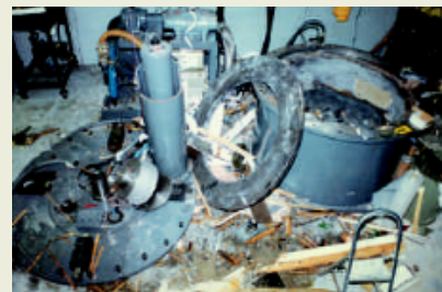
Figure 10.5.4 Some of the destruction caused by the explosion of a rapidly rotating steel disk.
