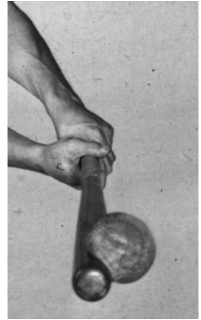
Figure 9.4.1 The collision of a ball with a bat collapses part of the ball.
