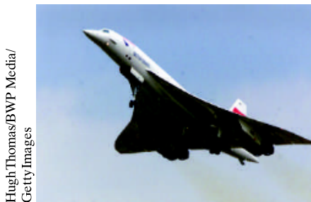
Figure 18.3.1 When a Concorde flew faster than the speed of sound, thermal expansion due to the rubbing by passing air increased the aircraft's length by about 12.5 cm. (The temperature increased to about 128^{\circ}\text{C} at the aircraft nose and about 90^{\circ}\text{C} at the tail, and cabin windows were noticeably warm to the touch.)
