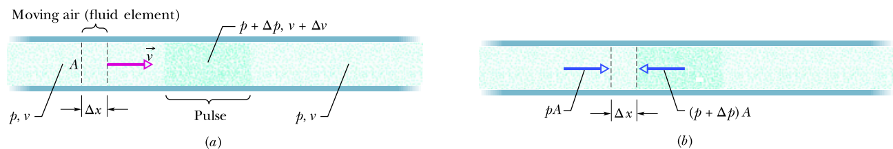
Figure 17.1.3 A compression pulse is sent from right to left down a long air-filled tube. The reference frame of the figure is chosen so that the pulse is at rest and the air moves from left to right. (a) An element of air of width \Delta x moves toward the pulse with speed v . (b) The leading face of the element enters the pulse. The forces acting on the leading and trailing faces (due to air pressure) are shown.
