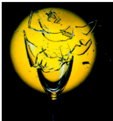
Sound can cause the wall of a drinking glass to oscillate. If the sound produces a standing wave of oscillations and if the intensity of the sound is large enough, the glass will shatter.
