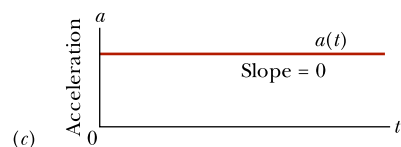
Figure 2.4.1 (a) The position x(t) of a particle moving with constant acceleration. (b) Its velocity v(t) , given at each point by the slope of the curve of x(t) . (c) Its (constant) acceleration, equal to the (constant) slope of the curve of v(t) .
