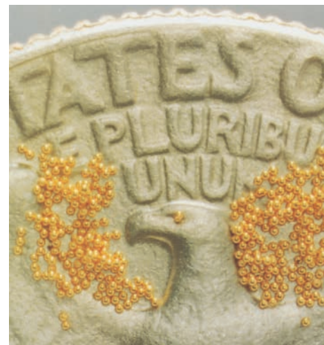
Figure 43-13 The small spheres on the quarter are deuterium–tritium fuel pellets, designed to be used in a laser fusion chamber.
