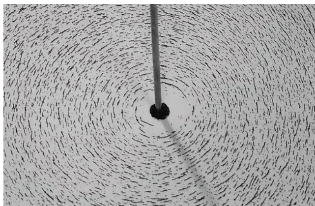
Figure 29-3 Iron filings that have been sprinkled onto cardboard collect in concentric circles when current is sent through the central wire. The alignment, which is along magnetic field lines, is caused by the magnetic field produced by the current.
