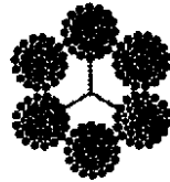
Fig. 3d. 6 × 41 Warrington-Seale with fiber core
