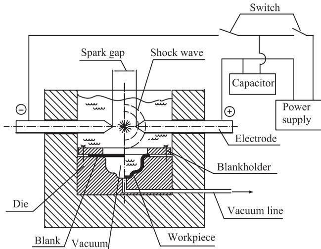
Fig. 32. Electrohydraulic Forming Set-up
