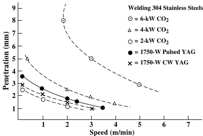
Fig. 11. Rates for CO<sub>2</sub> and Nd:YAG Laser Welding.
