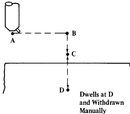
In the G88 dwell cycle, the tool is moved from A to B to C at the rapid traverse rate and then fed at the prescribed feed rate to D. The tool dwells at D, then stops rotating and is withdrawn manually.
