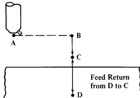
In the G85 boring cycle, the tool is moved from point A to point B and then to point C at the rapid traverse rate. The tool is next fed to point D and then, while still rotating, is moved back to point C at the same feed rate.
