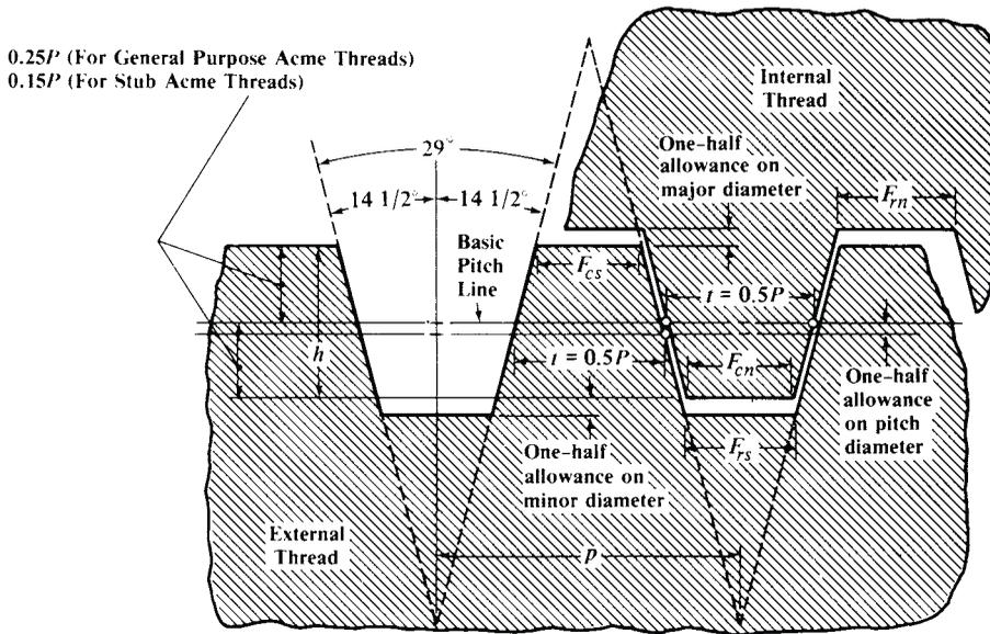
Fig. 1. General Purpose and Stub Acme Thread Forms
