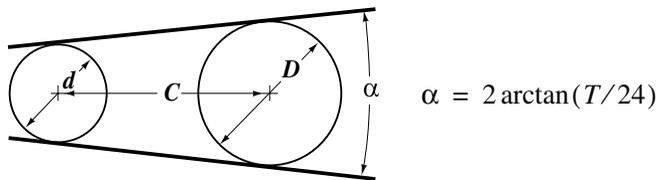
✿ *Example:* What angle  $\alpha$  is equivalent to a taper of 1.5 inches per foot?
