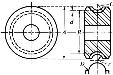
As the depth of the tooth is usually very slight, the throat diameter *B* will be accurate enough for all practical purposes for calculating the pitch, and it is not necessary to take into consideration the pitch circle. For example, assume that the pitch of a knurl is 32, that the throat diameter *B* is 0.5561 inch, that the radius *R* of the piece to be knurled is  $\frac{1}{16}$  inch, and that the angle of the teeth is 90 degrees; find the dimensions of the knurl. Using the notation given:
