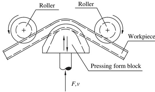
Fig. 66. Press Bending
