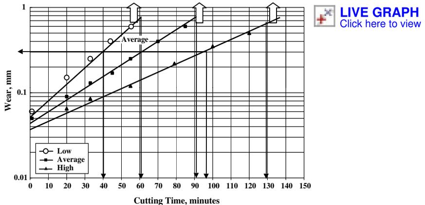
Fig. 1. Flank Wear as a Function of Cutting Time
