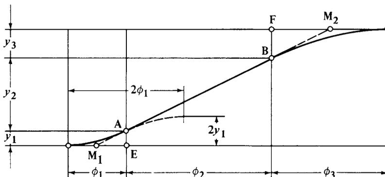
Fig. 9. Matching a Parabola at Each End of Straight Line Displacement Curve  $AB$  to Provide More Acceptable Acceleration and Deceleration
