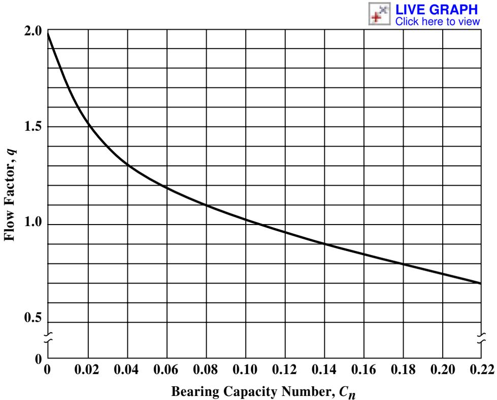
Fig. 10. Flow factor,  $q$ , vs. bearing capacity number,  $C_n$ —journal bearings.
