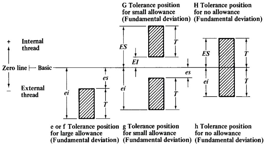
Fig. 5. Metric Tolerance System for Screw Threads
