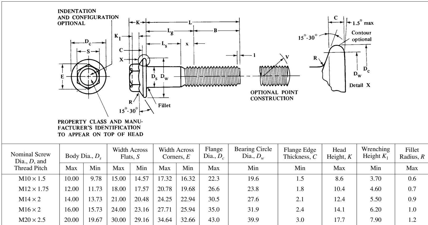
All dimensions are in millimeters. Basic thread lengths,  $B$ , are as given in Table 13. Transition thread length,  $x$ , includes the length of incomplete threads and tolerances on grip gaging length and body length. It is intended for calculation purposes. For additional manufacturing and acceptance specifications, reference should be made to ANSI/ASME B18.2.3.9M-1984 standard.
