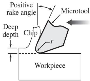
Fig. 2b. (b) Microfaceting, depth of cut  $> 0.5 r$ .
