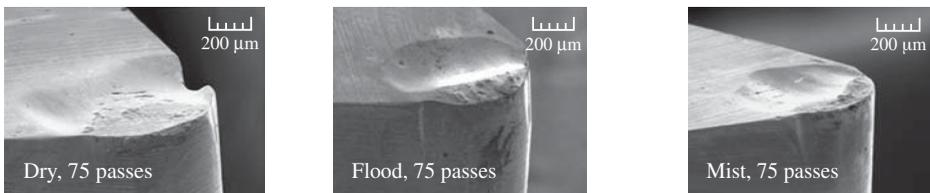
Fig. 30a. Dry machining. Fig. 30b. Rustlick 1:15 flood cooling. Fig. 30c. CL2210EP micromist.
