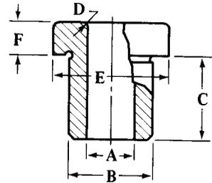
Fig. 6. Head Type Liner Bushings — Type HL
