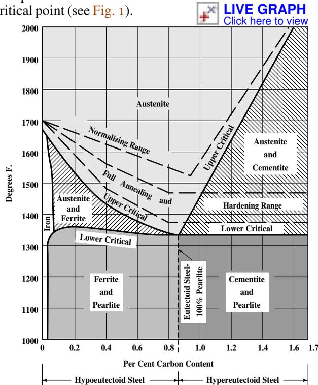
Fig. 1. Phase Diagram of Carbon Steel
