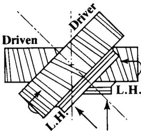
the two gears equals the shaft angle, and the gears are of the same hand, if each angle is less than the shaft angle. The difference between the helix angles equals the shaft angle, and the gears are of opposite hand, if either angle is greater than the shaft angle.
