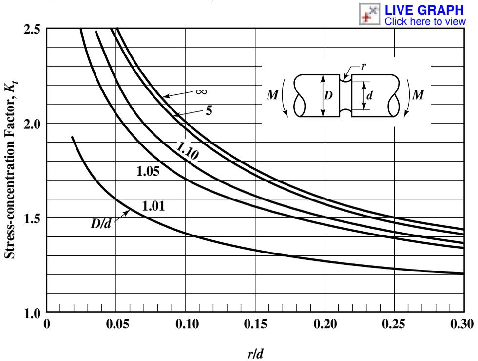
Fig. 8. Stress-concentration factor,  $K_t$ , for a grooved shaft in bending<sup>a</sup>
