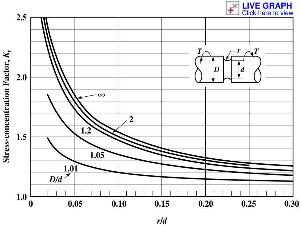
Fig. 9. Stress-concentration factor,  $K_t$ , for a grooved shaft in torsion<sup>a</sup>
