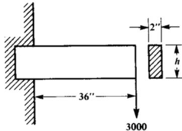
**Fig. 4. Determining the Depth  $h$  of a Beam to Support a Known Weight**
