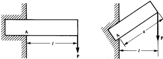
**Fig. 3. Diagrams Illustrating Principle of Bending Moments**
