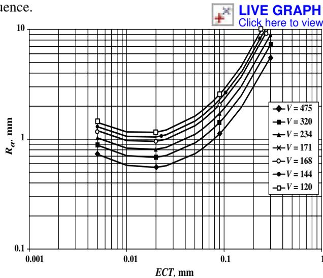
Fig. 13.  $R_a$  vs.  $ECT$ , nose radius  $r$  constant
