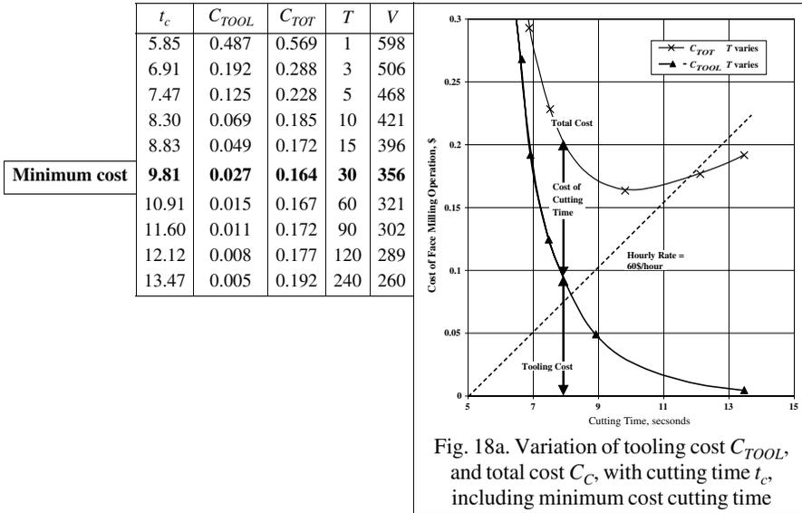
Fig. 18a. Variation of tooling cost  $C_{TOOL}$ , and total cost  $C_C$ , with cutting time  $t_c$ , including minimum cost cutting time
