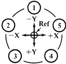
The diagram shows a type “A” circle for a 5-hole circle. Coordinates  $x$ ,  $y$  are given in the table for hole circles of from 3 to 28 holes. Dimensions are for holes numbered in a counterclockwise direction (as shown). Dimensions given are based upon a hole circle of unit diameter. For a hole circle of, say, 3-inch or 3-centimeter diameter, multiply table values by 3.
