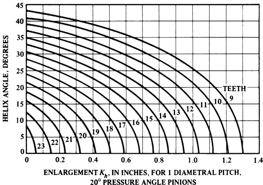
To eliminate the need for making the calculations indicated in **Formulas (3) and (4)**, the accompanying graph may be used to obtain the value of  $K_h$  directly for full-depth pinions of 20-degree normal pressure angle.
