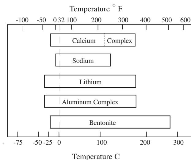
Fig. 10. Temperature Limit Guidelines for Grease
