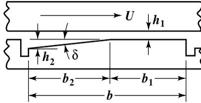
Fig. 7. Basic elements of tapered land thrust bearing.\*
