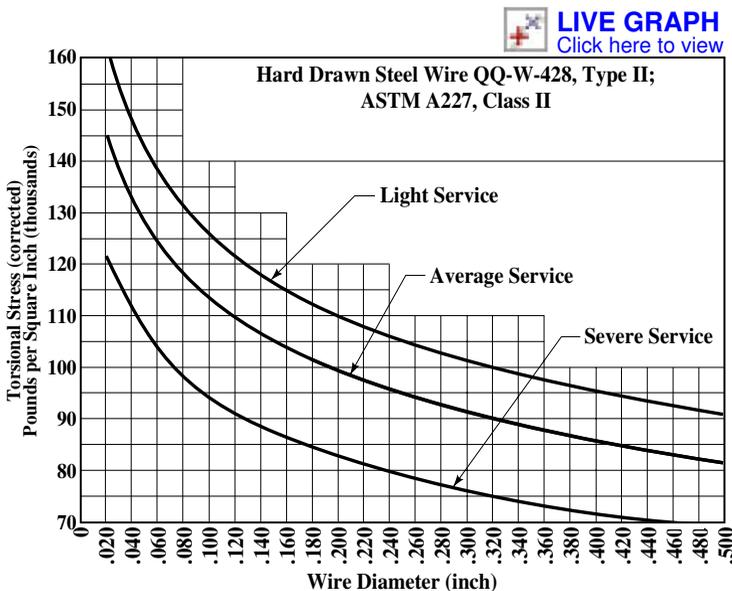
Fig. 1. Allowable Working Stresses for Compression Springs — Hard Drawn Steel Wire<sup>a</sup>
