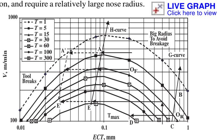
Fig. 7. Cutting speed vs. *ECT*, *V-ECT*, tool-life plotted
