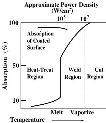
Fig. 5. Laser Energy Absorption Intensity vs. Temperature
