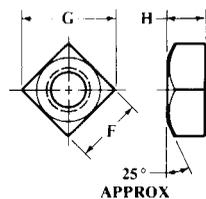
Fig. 10. Square Nuts, Heavy Square Nuts (Table 10)
