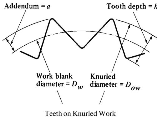
**Formulas Applicable to Knurled Work.**—The following formulas are applicable to knurled work with straight, diagonal, and diamond knurling.
