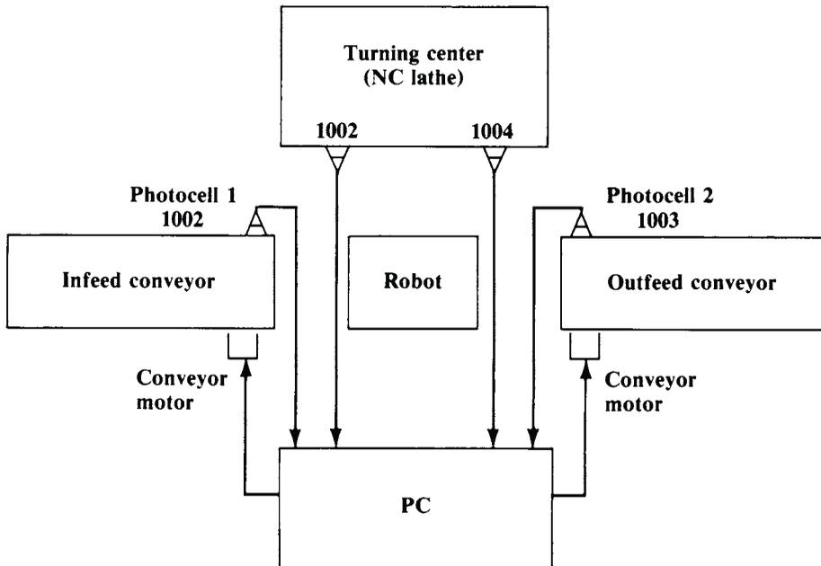
Fig. 3. Layout of a Flexible Manufacturing Module
