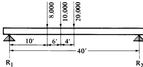
The sum of the reactions equals 38,000 pounds, which is also the sum of the loads. If part of the load is uniformly distributed over the beam, this part is first equally divided between the two supports, or the uniform load may be considered as concentrated at its center of gravity.
