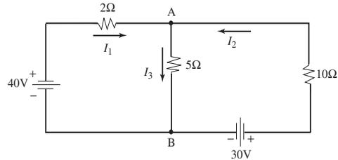
By combining all the above equations, a linear system of three independent equations is formed. Solve the system for the currents  $I_1, I_2$ , and  $I_3$ .
