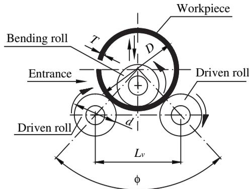
Fig. 17. Three-roll Bending
