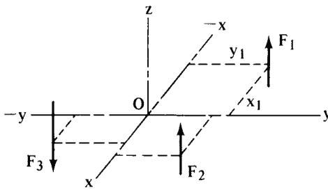
In the diagram, forces  $F_1, F_2,$  etc. represent a system of noncoplanar parallel forces. To find the resultant of such systems, use the procedure shown below.
