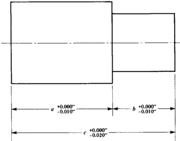
Fig. 7. One Interpretation of Dimensioning in Fig. 6
