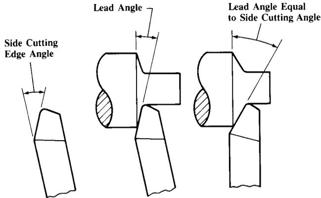
Fig. 2. Lead Angle on Single-point Turning Tool
