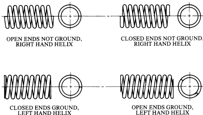
Fig. 12. Types of Helical Compression Spring Ends
