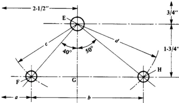
**Fig. 14. Find Dimensions a, b, c, and d**
