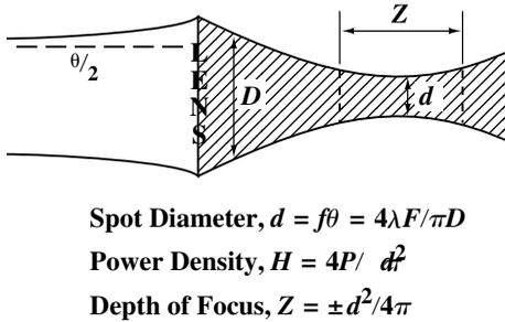
Fig. 3. Focus Characteristics of a Laser Beam.
