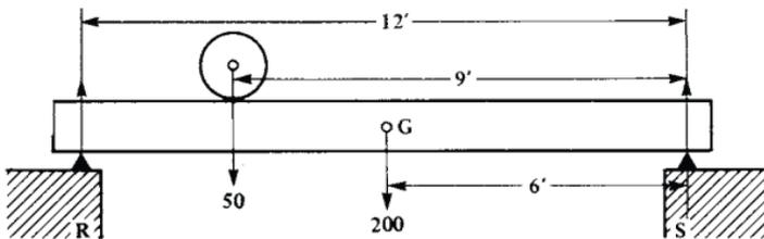
**Fig. 3. The Weight on Each Support is Required**
