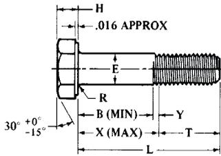
Fig. 2. Heavy Hex Structural Bolts (Table 2)
