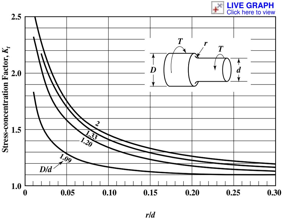
Fig. 5. Stress-concentration factor,  $K_t$ , for a filleted shaft in torsion<sup>a</sup>
