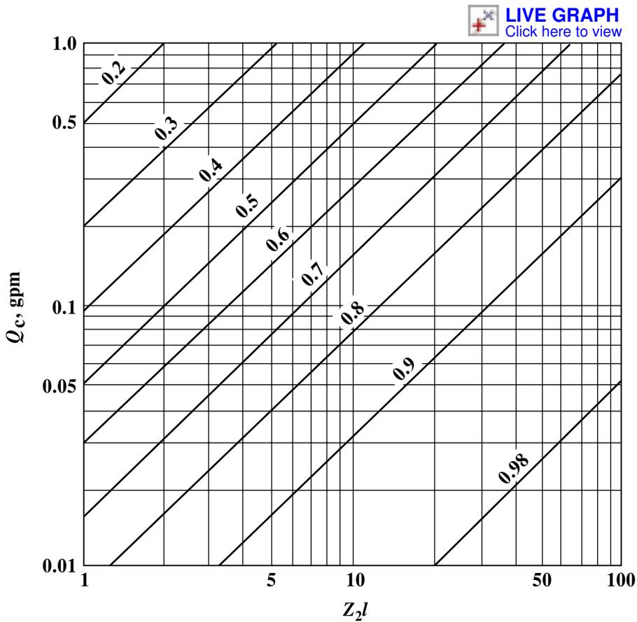
Fig. 4. Kinetic energy correction factor,  $\xi$ —thrust bearings.<sup>a</sup>
