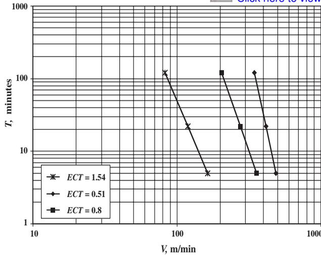
Fig. 20b. Tool-life vs. cutting speed, constant ECT
