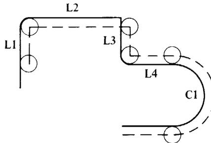
Fig. 3. Motion Statements for Movements Around a Workpiece
