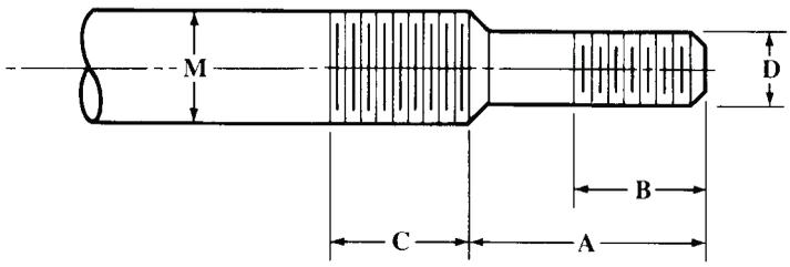
The diagram shows a side view of a draw-in bolt end. It consists of a large diameter section on the left, a section of usable thread of length C, a section of unusable thread of length B, and a small diameter section of length A. The diameter of the large end is M, and the diameter of the small end is D.
