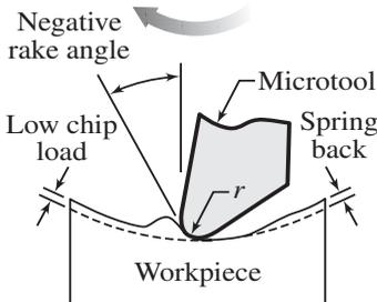
Fig. 2c. (c) Micromilling, chip load  $< 0.5 r$ .
