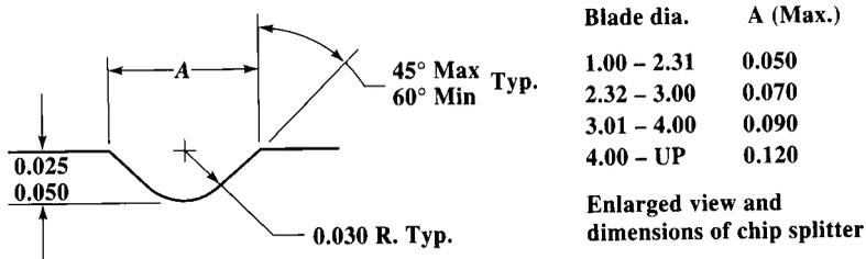
Fig. 4. Spade Drill Chip Splitter Dimensions in Inches
