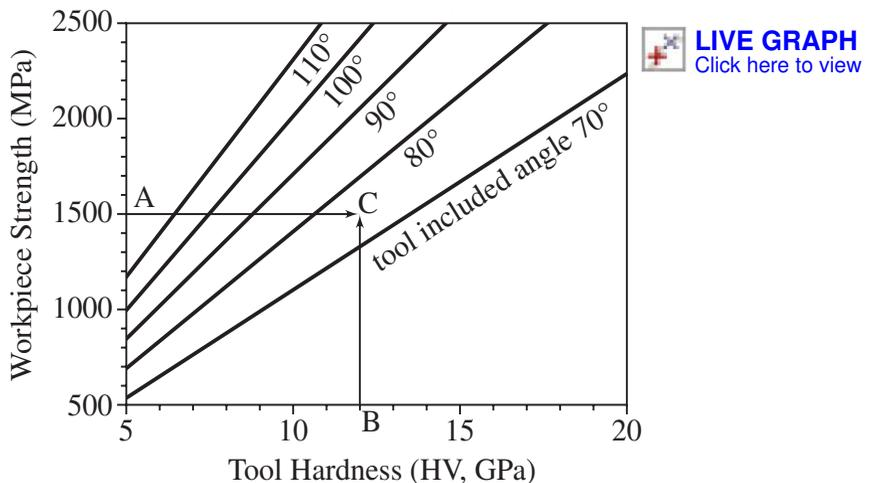
Fig. 5. Microtool minimum included angles.
