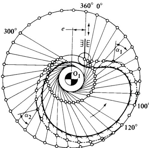
Fig. 16. Construction of Cam Contour; Offset Translating Follower
