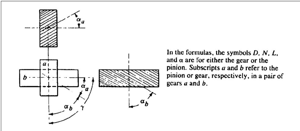
In the formulas, the symbols  $D$ ,  $N$ ,  $L$ , and  $\alpha$  are for either the gear or the pinion. Subscripts  $a$  and  $b$  refer to the pinion or gear, respectively, in a pair of gears  $a$  and  $b$ .
