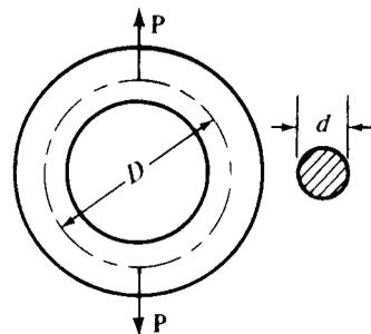
The *decrease* in the horizontal diameter will be about 92% of the increase in the vertical diameter given by **Formula (26)**. In the above formulas,  $P$  = load on ring in pounds;  $D$  = mean diameter of ring in inches;  $S$  = tensile stress in pounds per square inch,  $I$  = moment of inertia of section in inches<sup>4</sup>; and  $E$  = modulus of elasticity of material in pounds per square inch.
