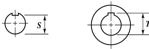
**Table 2. Depth Control Values S and T for Shaft and Hub**
