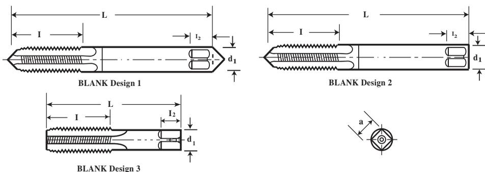
**Table 5a. Standard Tap Dimensions (Ground and Cut Thread) ASME B94.9-1999**
