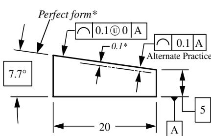
Fig. 10c. Internal Unilateral Tolerance Zone About Perfect Form.
