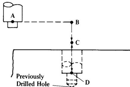
This G82 code produces a cycle that is very similar to the cycle of the G81 code except for the dwell period at point D. The dwell period allows the tool to smooth out the bottom of the counterbore or spotface. The time for the dwell, in seconds, is noted as a T-word.
