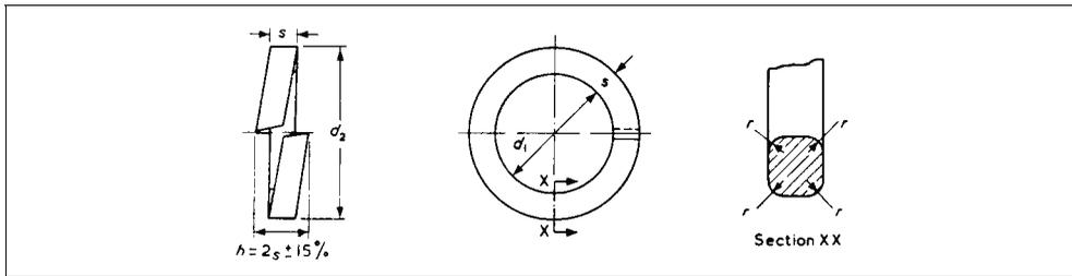
**British Standard Single Coil Square Section Spring Washers; Metric Series —
