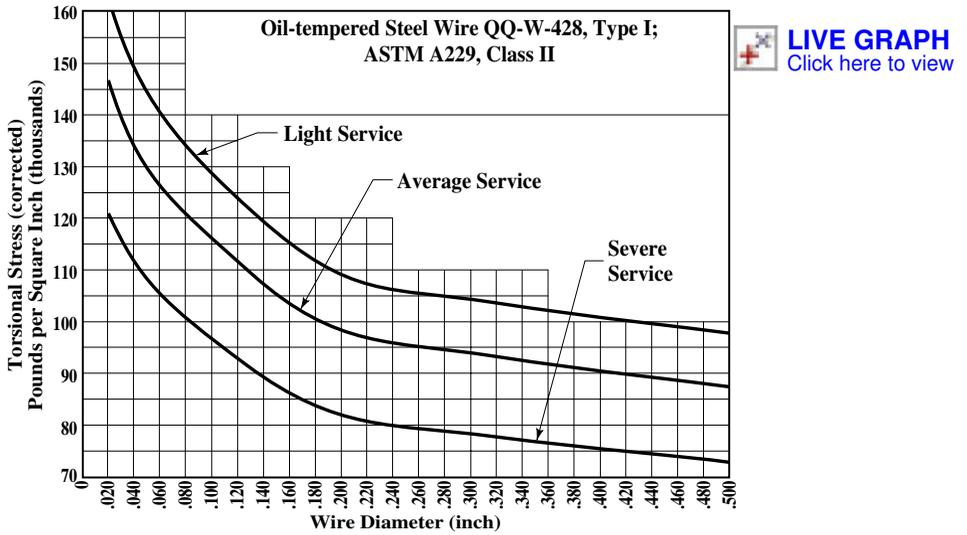
Fig. 3. Allowable Working Stresses for Compression Springs — Oil-Tempered<sup>a</sup>
