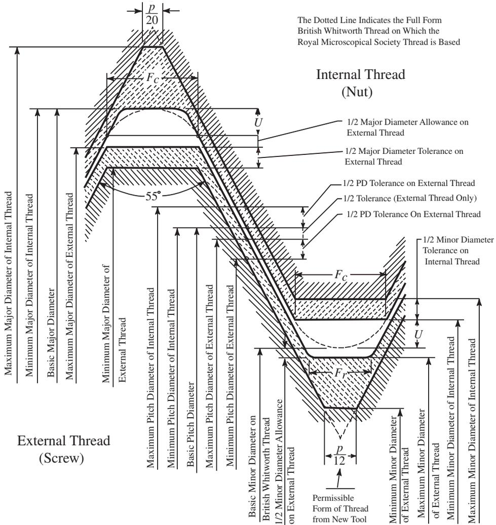
Tolerances, Allowances and Crest Clearances for Microscope Objective Thread (AMO)
