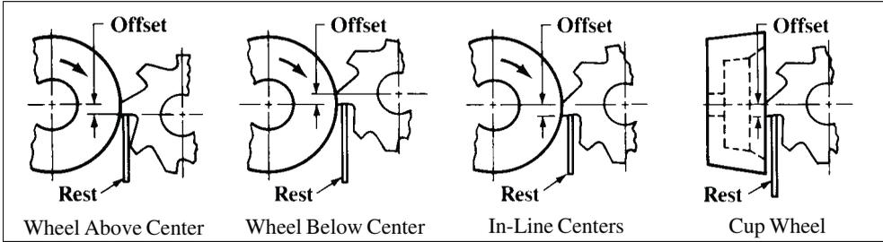
**Distance to Set Center of Wheel Above the Cutter Center (Disk Wheel)**
