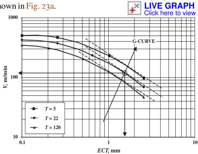
Fig. 23a. Cutting speed vs. ECT, tool-life constant
