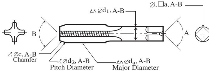
**Table 15. Tap Thread Limits: Metric Sizes, Ground Thread
