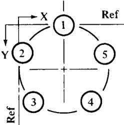
The diagram shows a type “A” circle for a 5-hole circle. Coordinates  $x$ ,  $y$  are given in the table for hole circles of from 3 to 28 holes. Dimensions are for holes numbered in a counterclockwise direction (as shown). Dimensions given are based upon a hole circle of unit diameter. For a hole circle of, say, 3-inch or 3-centimeter diameter, multiply table values by 3.
