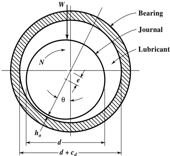
Fig. 1. Basic components of a journal bearing.
