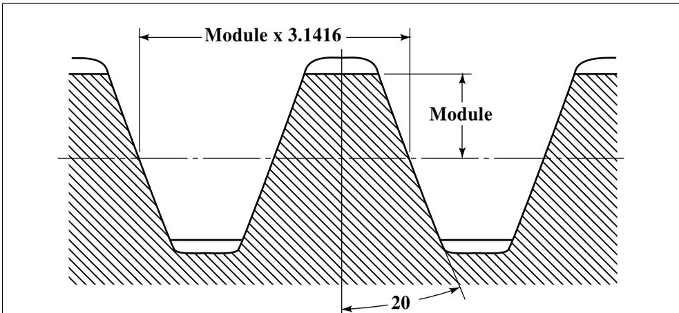
The flanks or sides are straight (involute system) and the pressure angle is 20 degrees. The shape of the root clearance space and the amount of clearance depend upon the method of cutting and special requirements. The amount of clearance may vary from 0.1 × module to 0.3 × module.
