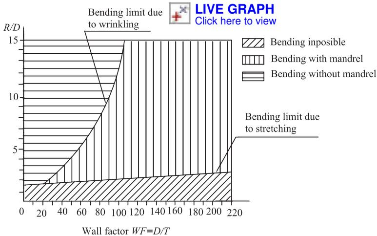
Fig. 65. Technical Limits of the Tube/pipe Bending Process
