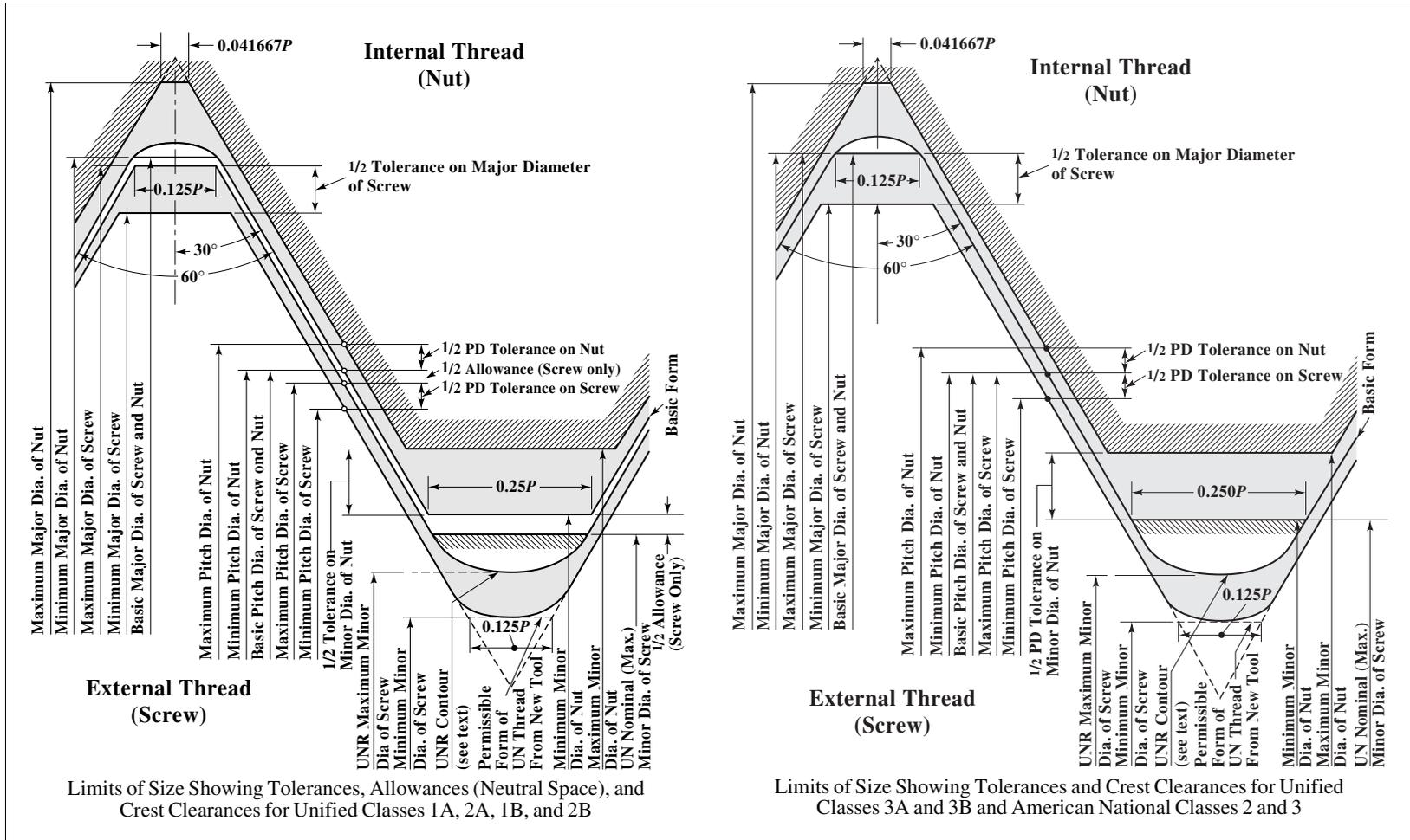
ance provides adequate undercut for such coatings. There may be variations in thickness and symmetry of coating resulting from commercial processes but after plating the threads should be accepted by a basic Class 3A size GO gage and a Class 2A gage as a NOT-GO gage. Class 1A provides an allowance which is maintained for both coated and uncoated product, i.e., it is not available for coating.
