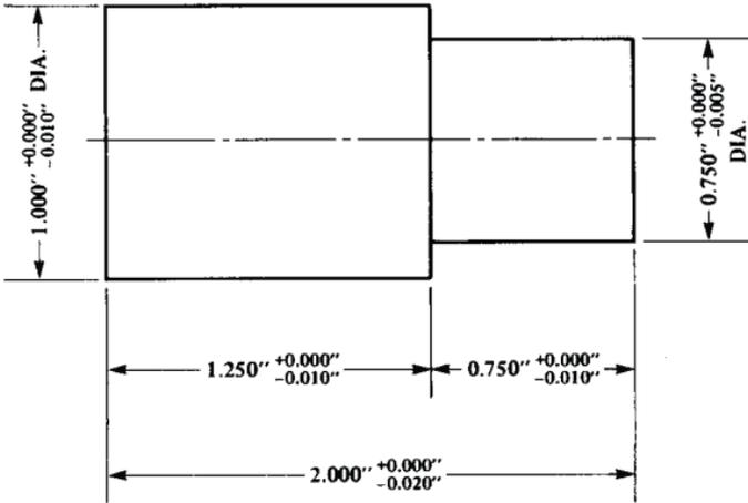
Fig. 6. Common but Incorrect Method of Dimensioning
