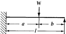
$N = 775,200 \frac{d^2 l}{ab} \sqrt{\frac{l}{Wa(3l+b)}}$ <p>One-fixed — One supported</p>      |
