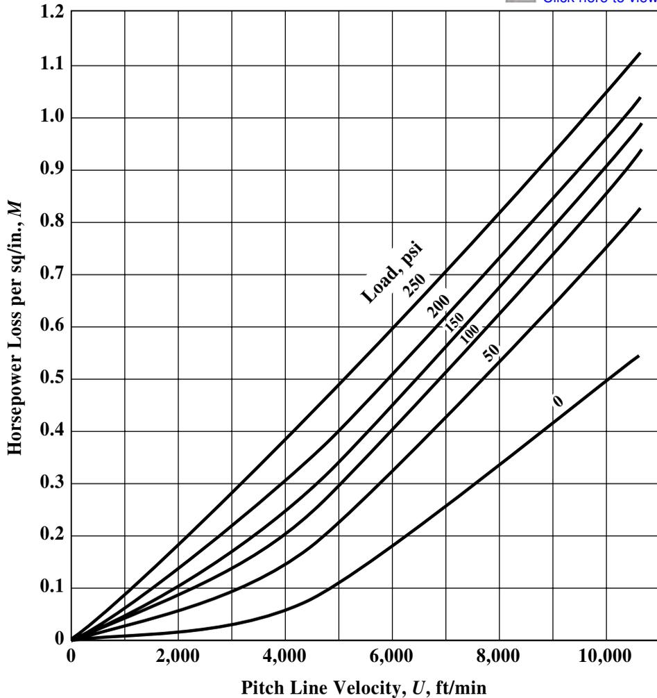
Fig. 3. Friction power loss,  $M$ , vs. peripheral speed,  $U$  — thrust bearings.<sup>a</sup>
