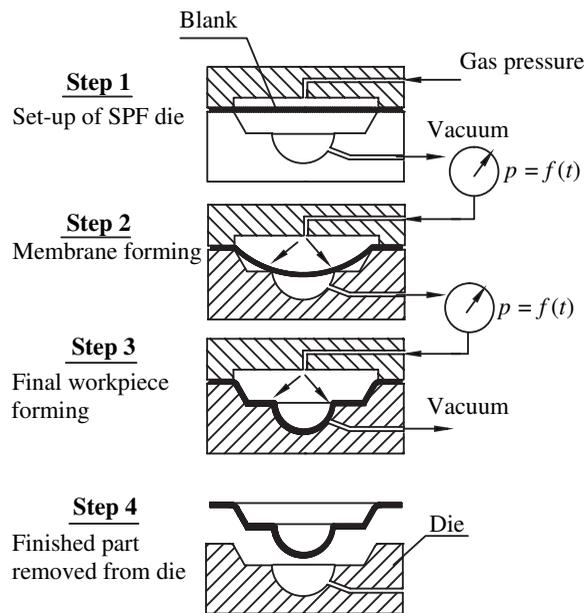
Fig. 27. Schematic Illustration of Superplastic Forming Process
