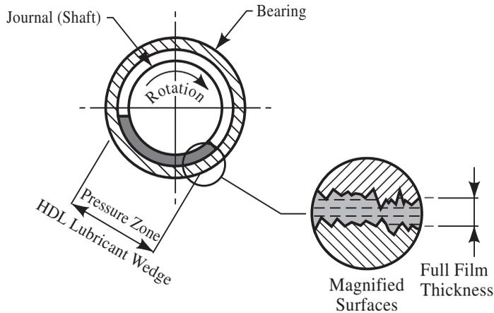
Fig. 2. HDL Hydrodynamic Lubrication of a Journal Bearing
