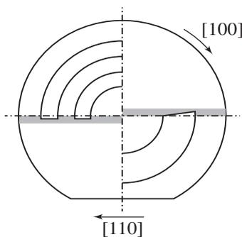
Fig. 14. Machining plan on (001) wafers. A wafer was faced at a constant depth in different zones (left) or changing cutting depth in a taper cut (right).
