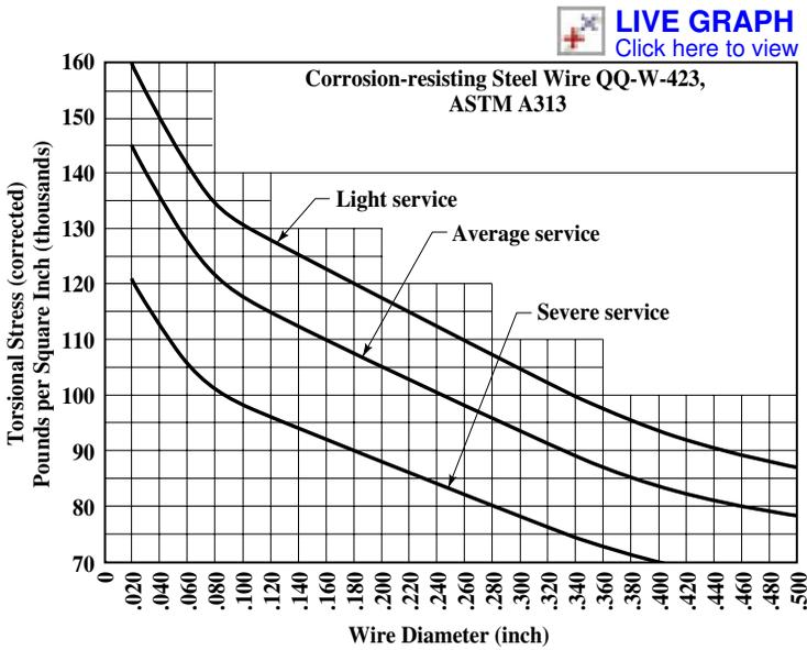
Fig. 5. Allowable Working Stresses for Compression Springs — Corrosion-Resisting Steel Wire<sup>a</sup>
