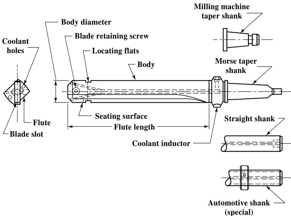
Fig. 1. Spade Drill Blade Holder
