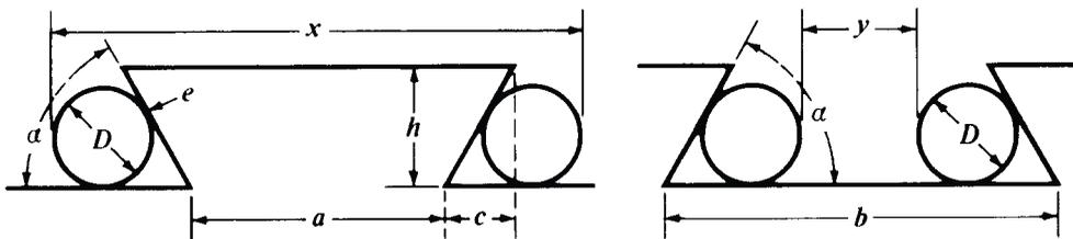
The rod or wire used should be small enough so that the point of contact *e* is somewhat below the corner or edge of the dovetail.
