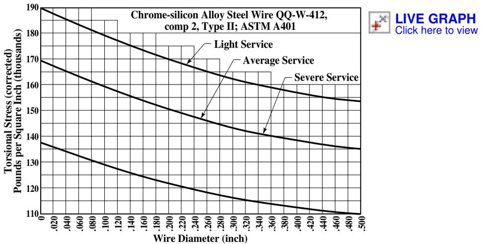
Fig. 4. Allowable Working Stresses for Compression Springs — Chrome-Silicon Alloy Steel Wire<sup>a</sup>
