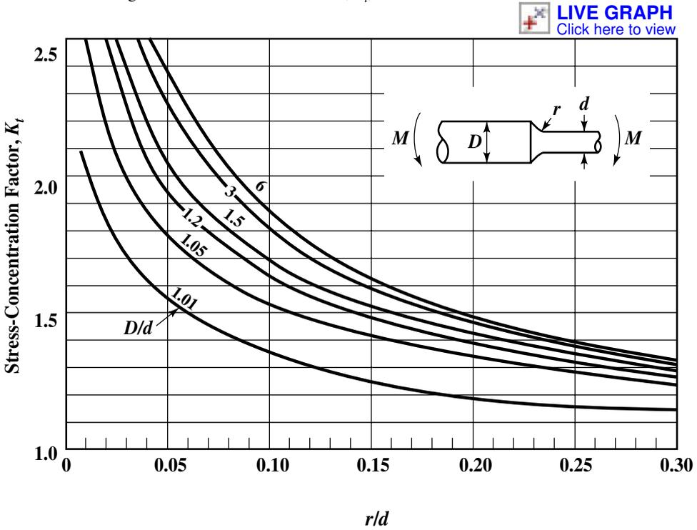
Fig. 6. Stress-concentration factor,  $K_t$ , for a shaft with shoulder fillet in bending<sup>a</sup>
