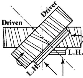
**5. Shafts at Any Angle, Center Distance Approximate.**— The sum of the helix angles of the two gears equals the shaft angle, and the gears are of the same hand, if each angle is less than the shaft angle. The difference between the helix angles equals the shaft angle, and the gears are of opposite hand, if either angle is greater than the shaft angle.
