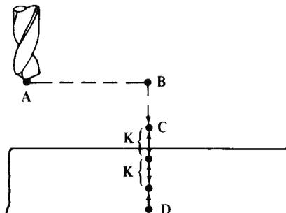
In the G83 peck-drilling cycle, the drill is moved from point A to point B and then to point C at the rapid traverse rate; the drill is then fed the incremental distance K, followed by
