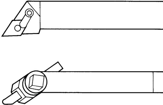
Fig. 3. Top: Right-hand Offset-shank, Indexable Insert Holder
