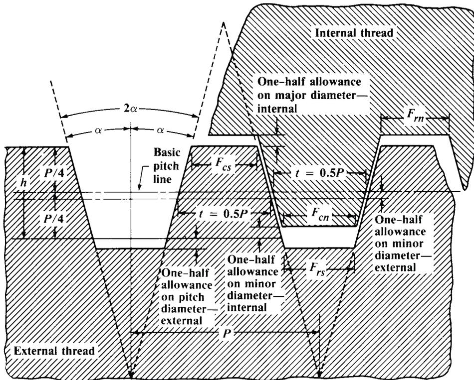
Fig. 3. Centralizing Acme Screw Thread Form
