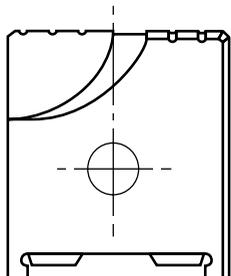
Fig. 2d. Center cutting facing or bottoming blade
