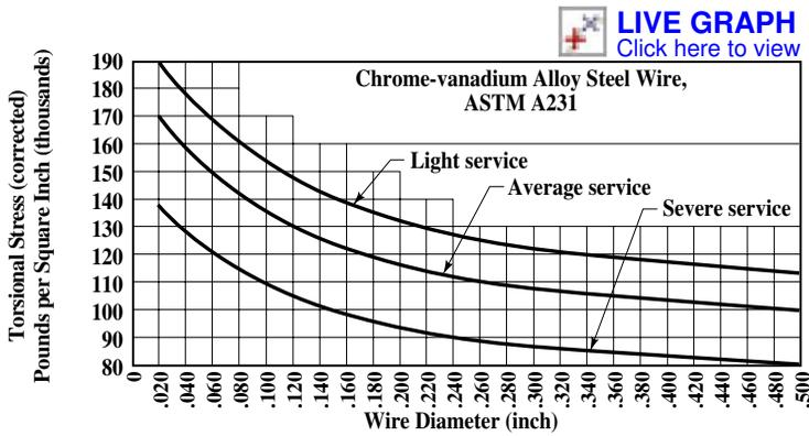
Fig. 6. Allowable Working Stresses for Compression Springs — Chrome-Vanadium Alloy Steel Wire<sup>a</sup>
