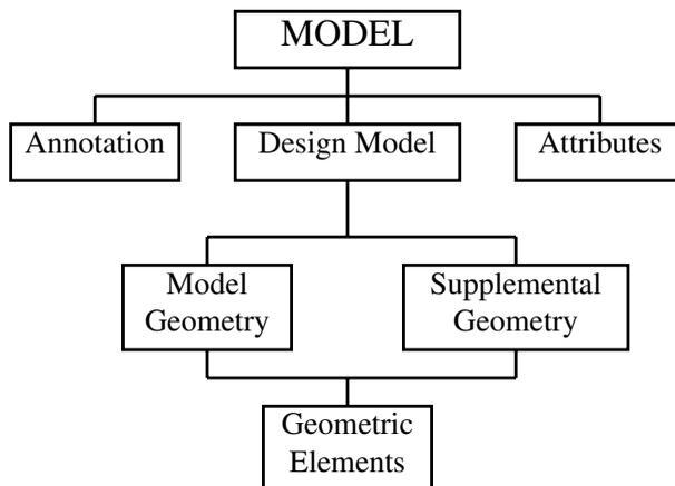
Fig. 16. Content of a Digital Model (ANSI Y14.41-2003).
