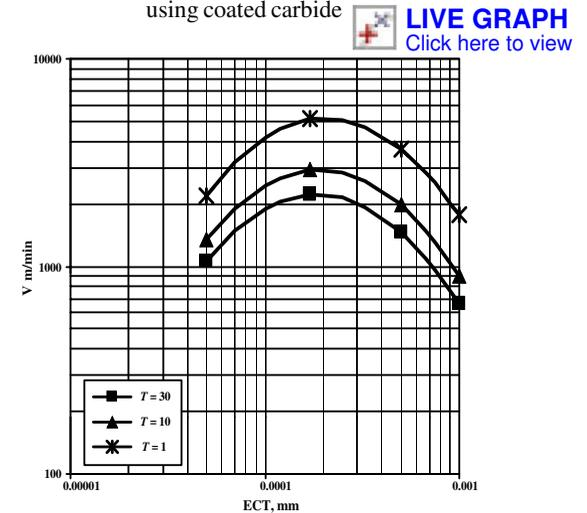
Fig. 17h. Wheel-life in grinding M4 tool-steel
