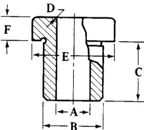
Fig. 4. Fixed Type Renewable Wearing Bushings — Type F
