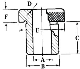
Fig. 3. Slip Type Renewable Wearing Bushings — Type S
