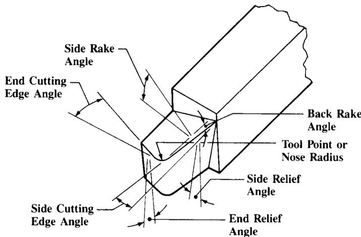
Fig. 1. Terms Applied to Single-point Turning Tools
