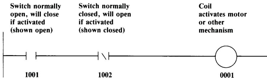
Fig. 2. One Rung on a Ladder Diagram
