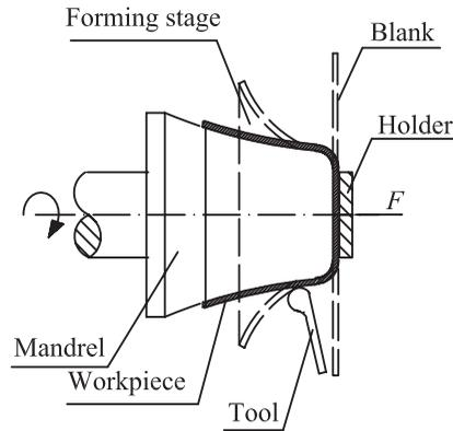
Fig. 22. Conventional Spinning
