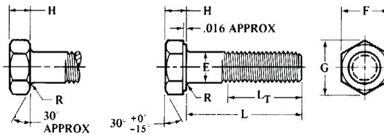
Fig. 4. Hex Cap Screws, Heavy Hex Screws (Table 4)
