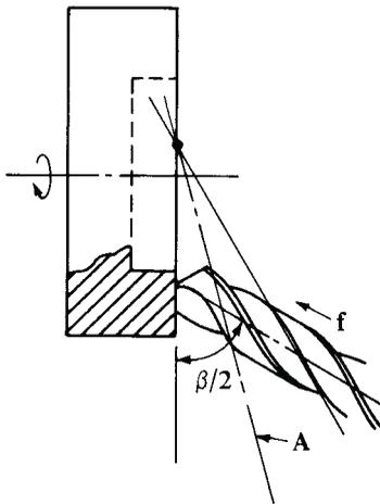
Fig. 2. In grinding the face of the twist drill the tool is swung around the axis  $A$  of an imaginary cone, while resting in a support tilted by half of the point angle  $\beta$  with respect to the face of the grinding wheel. Feed  $f$  for stock removal is in the direction of the drill axis.
