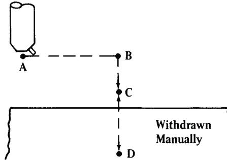
In the G87 canned boring cycle, the cutting tool is moved from A to B and then to C at the rapid traverse rate. The tool is then fed to D. The cycle is identical to the other boring cycles except that the tool is withdrawn manually.
