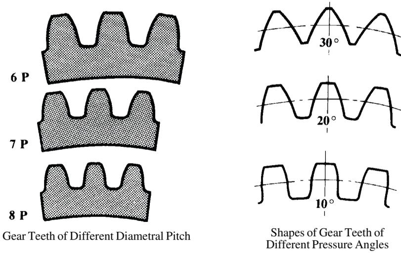
Gear Teeth of Different Diametral Pitch
