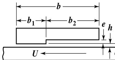
Fig. 6. Basic elements of step thrust bearing.\*
