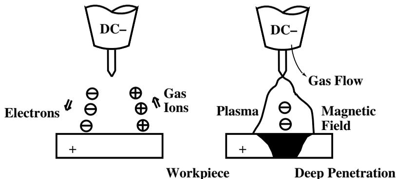
Fig. 8. Straight Polarity (DC<sup>-</sup>) Provides Highest Electrode Current Capacity and Deepest Penetration Potential.
