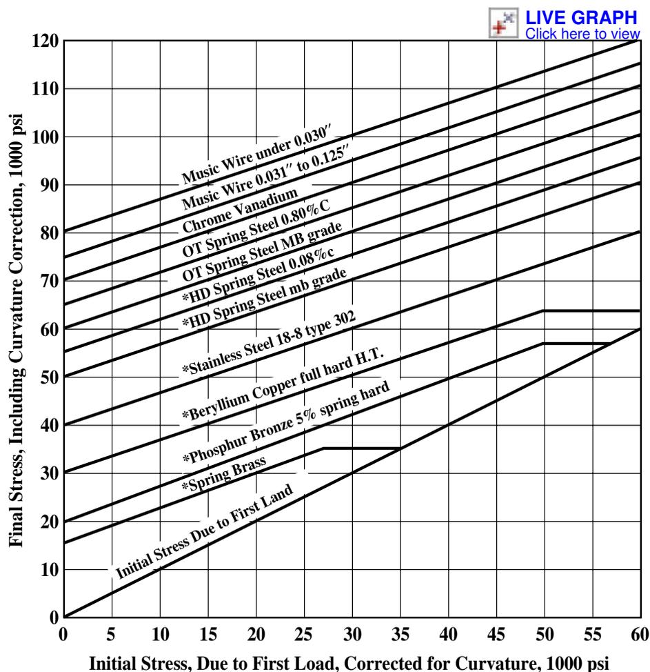
Fig. 11. Endurance Limit Curves for Compression Springs
