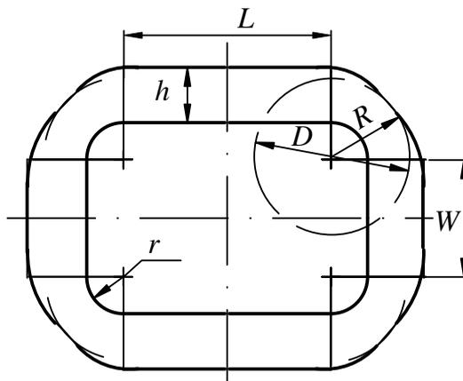
Fig. 18. Layout Design for Deep Drawn Rectangular Shell
