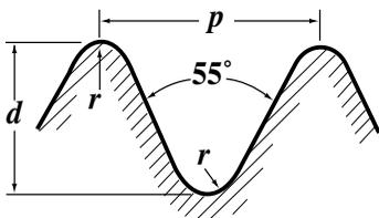
It is recommended that stainless steel bolts of nominal size  $\frac{3}{4}$  inch and below should not be made to Close Class limits but rather to Medium or Free Class limits. Nominal sizes above  $\frac{3}{4}$  inch should have maximum and minimum limits 0.001 inch smaller than the values obtained from the table.
