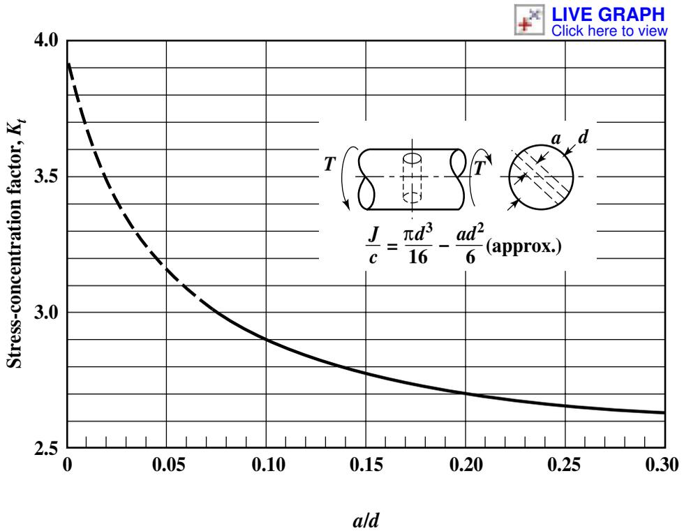
Fig. 7. Stress-concentration factor,  $K_t$ , for a shaft, with a transverse hole, in torsion<sup>a</sup>
