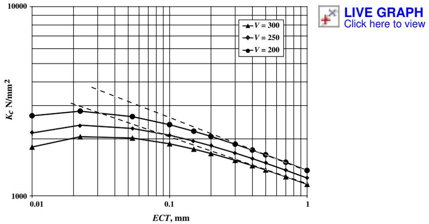
Fig. 9.  $K_c$  vs.  $ECT$ , cutting speed plotted
