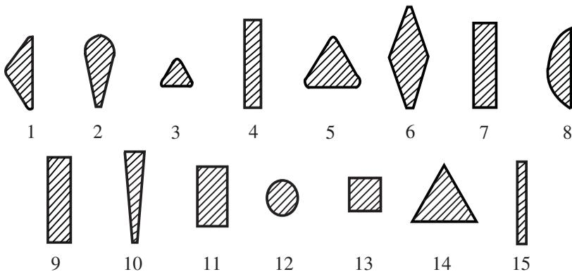
Fig. 1. Styles of Mill or Saw Files
