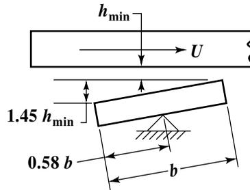
Fig. 12. Basic elements of tilting pad thrust bearing.\*
