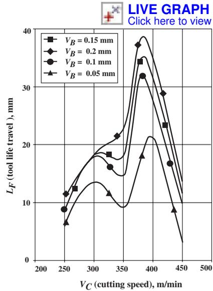
Fig. 3. Influence of cutting speed on tool-life
