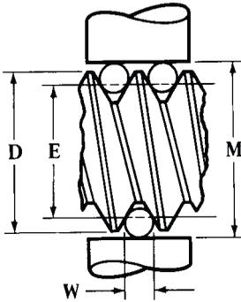
The formulas below do not compensate for the effect of the lead angle upon measurement  $M$ , but they are sufficiently accurate for checking standard single-thread screws unless exceptional accuracy is required. See accompanying information on effect of lead angle; also matter relating to measuring wire sizes, accuracy required for such wires, and contact or measuring pressure.
