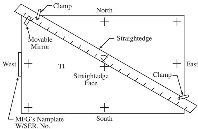
Fig. 6. Placement of the straightedge for measurement of the first reference line
