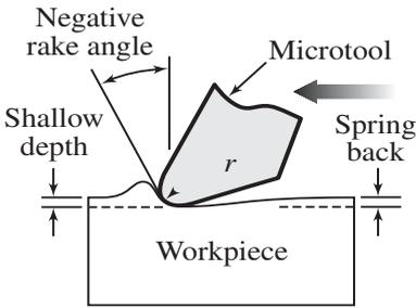
Fig. 2a. (a) Microfaceting, depth of cut  $< 0.5 r$ .
