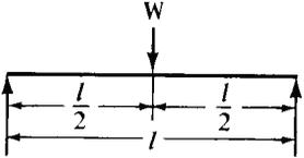
$N = 1,550,500 \frac{d^2}{l\sqrt{Wl}}$ <p>Bearings supported</p>                               |
