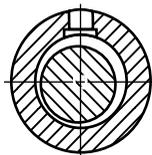
Fig. 3d. Straight axial groove with feeder groove
