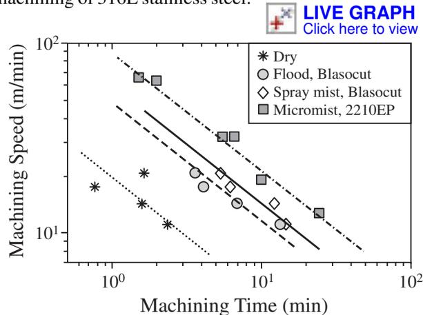
Fig. 27. Effect of cutting fluid conditions on micromilling of 316L stainless steel.  $10\mu\text{m}$ /tooth chip load,  $0.348\text{ mm}$  axial depth,  $0.558\text{ mm}$  radial depth,  $\text{Ø}1\text{ mm}$  uncoated carbide tool.
