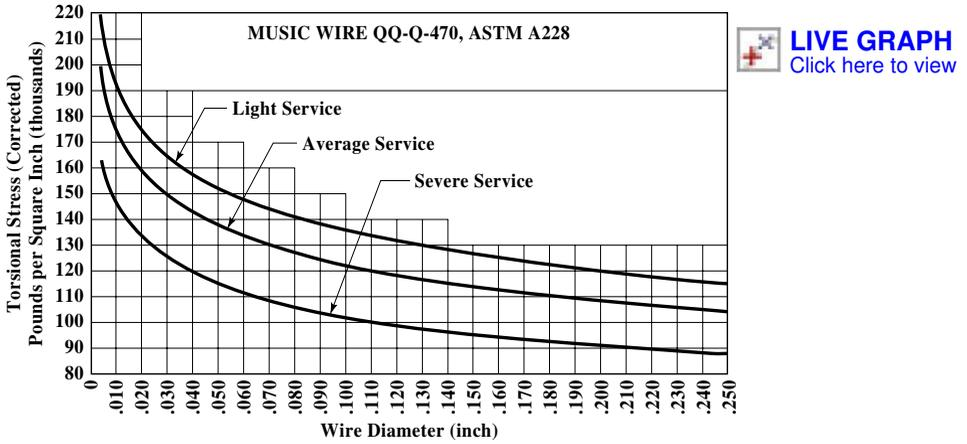
Fig. 2. Allowable Working Stresses for Compression Springs — Music Wire<sup>a</sup>
