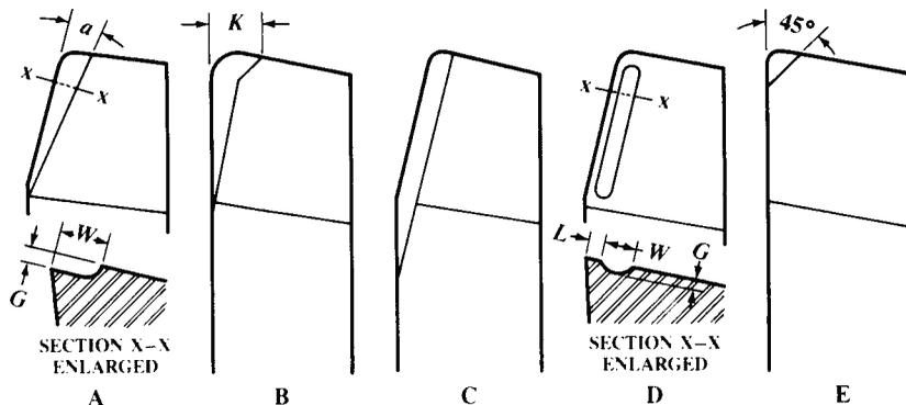
Fig. 4. Different Forms of Chipbreakers for Turning Tools
