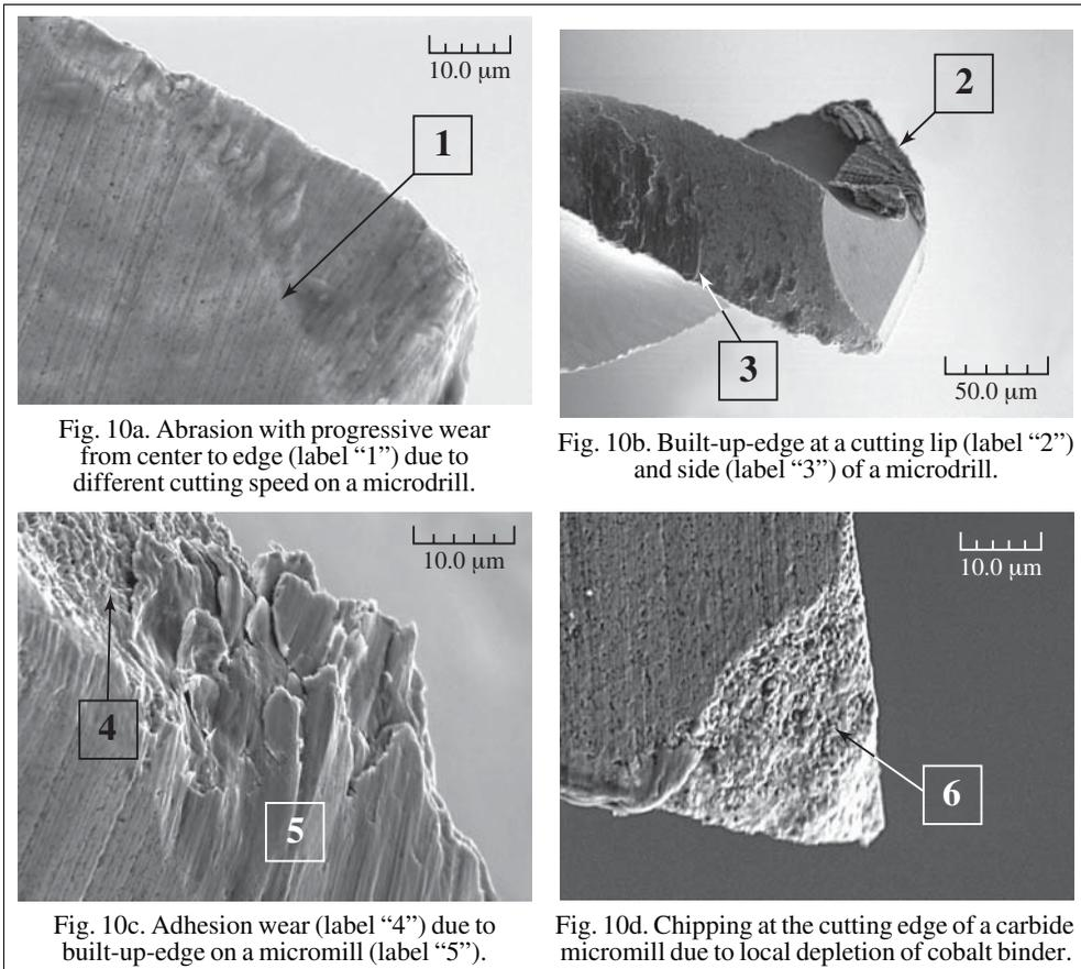
*Thermal effect* is the second cause of tool damage. A cutting tool edge is softened at high machining temperature, deformed plastically, and removed from the tool. Both high speed steel tools and carbide tools with high cobalt content are vulnerable to thermal damage. High temperature also promotes diffusion, i.e., atoms from the tool and workpiece move
