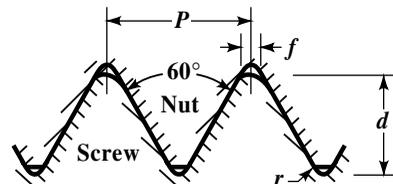
*International Metric Fine Thread:* The International Metric Fine Thread form of thread is the same as the International system but the pitch for a given diameter is smaller.
