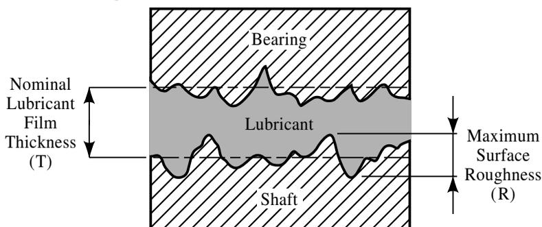
Fig. 1. Determining the Working Film Thickness Ratio Lambda
