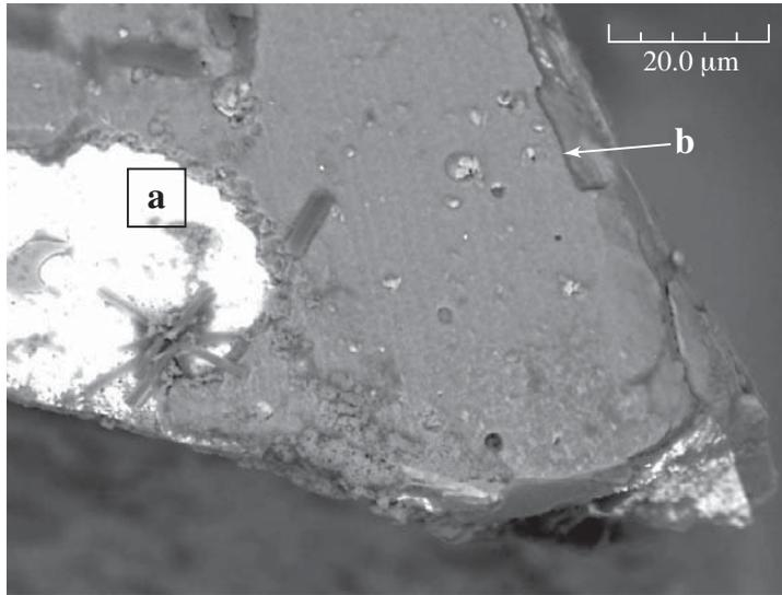
Fig. 6. Peeling (a) and cracking (b) of 4 $\mu$ m-thick TiN coating layer on a WC micromill. Back scattered electron technique shows high contrast of a dark TiN coating layer against the bright WC/Co substrate in the background.
