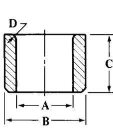
Fig. 5. Headless Type Liner Bushings — Type L
