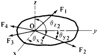
To find the resultant of any number of noncoplanar concurrent forces  $F_1, F_2, F_3$ , etc., use the procedure outlined below.
