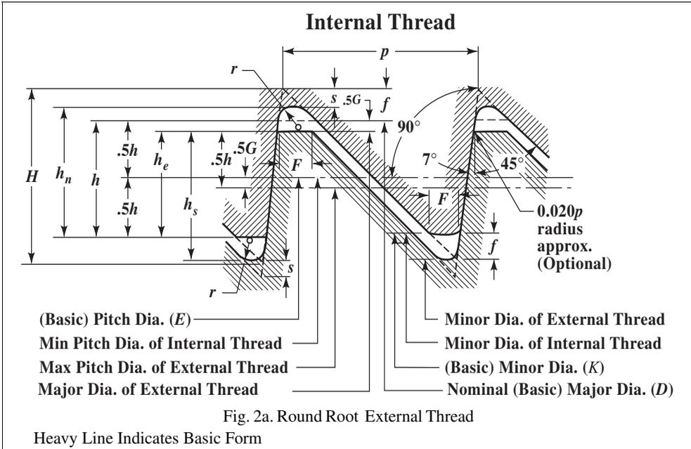
Fig. 2a. Round Root External Thread
