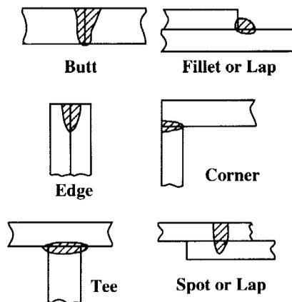
Fig. 10. Examples of Laser Weld Joint Designs.
