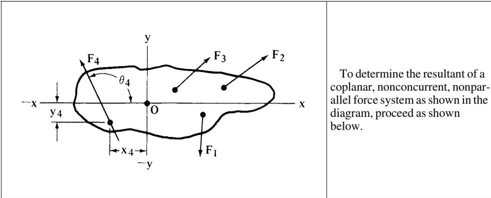
To determine the resultant of a coplanar, nonconcurrent, nonparallel force system as shown in the diagram, proceed as shown below.
