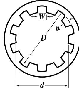
Fig. 7c. 10-Spline Fitting
