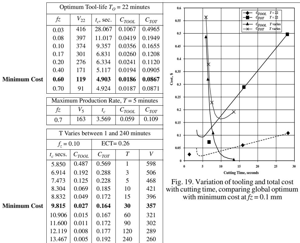
Fig. 19. Variation of tooling and total cost with cutting time, comparing global optimum with minimum cost at  $f_z = 0.1$  mm
