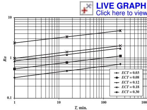
Fig. 16.  $R_a$  vs.  $T$ , holding  $ECT$  constant
