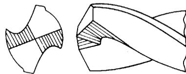
Fig. 4. Split point or "crankshaft" type web thinning.
