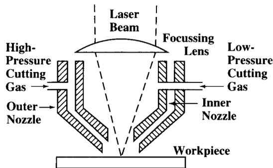
Fig. 7. Laser Gas Cutting Nozzle for Steel.
