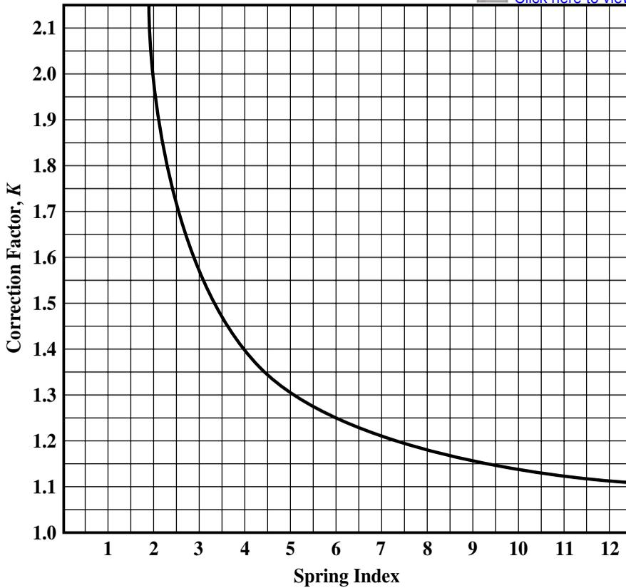
Fig. 13. Compression and Extension Spring-Stress Correction for Curvature<sup>a</sup>
