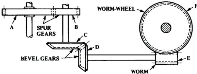
**Fig. 2. Combination of Spur, Bevel, and Worm Gearing**
