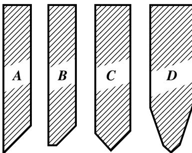
Fig. 63. Cutting Edges for Steel Rule Dies
