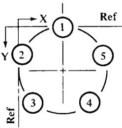
The diagram shows a type “A” circle for a 5-hole circle. Coordinates x, y are given in the table for hole circles of from 3 to 28 holes. Dimensions are for holes numbered in a counterclockwise direction (as shown). Dimensions given are based upon a hole circle of unit diameter. For a hole circle of, say, 3-inch or 3-centimeter diameter, multiply table values by 3.
