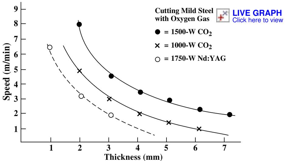
Fig. 8. Typical Cutting Rates for CO<sub>2</sub> and YAG Lasers.
