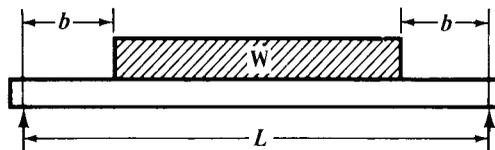
If the formulas are used with metric SI units,  $W$  = total load in newtons;  $L$  = total length between supports in millimeters;  $E$  = modulus of elasticity in newtons per millimeter<sup>2</sup>;  $I$  = moment of inertia of beam section in millimeters<sup>4</sup>;  $a$  = fraction of length of beam at each end, that is not loaded =  $b \div L$ ; and  $f$  = deflection in millimeters. The bending moment  $M_{\max}$  is in newton-millimeters (N · mm).
