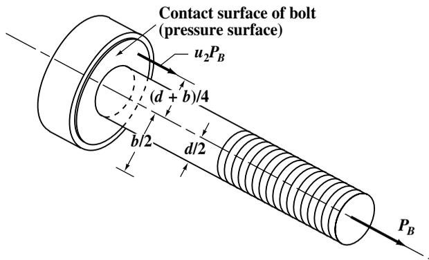
Fig. 7. Nut or Bolt Head Friction Force
