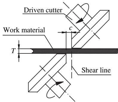
Fig. 4. Schematic Illustration of Shearing with Rotary Cutters
