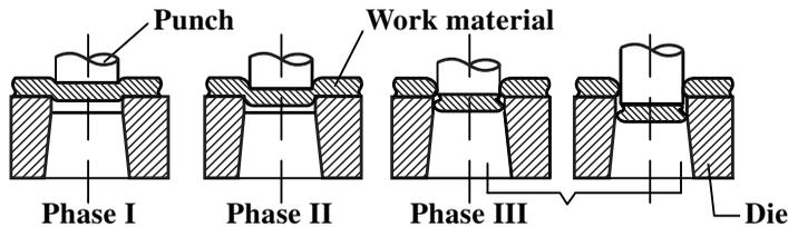
Fig. 8. Phases in the Process of Shearing
