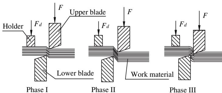
Fig. 3. Schematic Illustration of the Phases of Shearing
