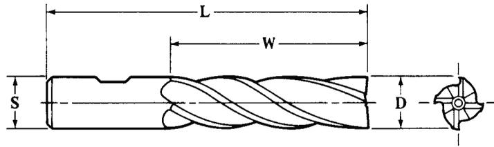
As Indicated By The Dimensions Given Below, Shank Diameter S May Be Larger, Smaller, Or The Same As The Cutter Diameter D
