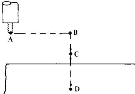
The G84 canned tapping cycle starts with the end of the tap being moved from point A to point B and then to point C at the rapid traverse rate. The tap is then fed to point D, reversed, and moved back to point C.
