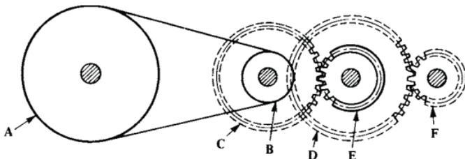
**Fig. 1. Combination Pulley and Compound Gear Drive**
