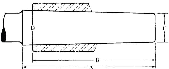
$$D = \frac{\text{no. of taper}}{8} \quad C = \frac{\text{no. of taper}}{10} \quad B = \frac{\text{no. of taper}}{2}$$
