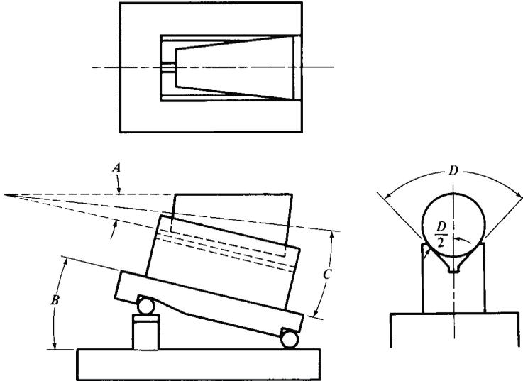
The sine-bar is set to angle  $B = (C + A/2)$  where  $A/2$  is one-half the included angle of the tapered part. If  $D$  is the included angle of the precision vee-block, the angle  $C$  is calculated from the formula:
