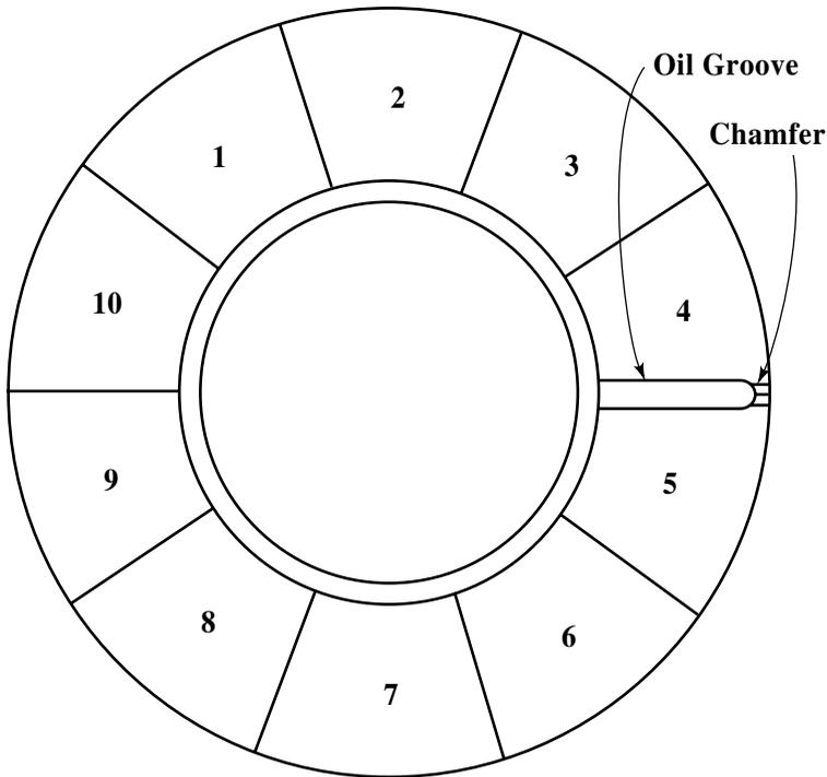
Fig. 5. Flat plate thrust bearing example design.\*
