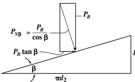
Fig. 5. Free Body Diagram of Thread Helix Forces
