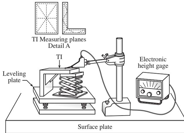
Fig. 8. Measuring Flatness/Parallelism of Type III Right-angle Plate
