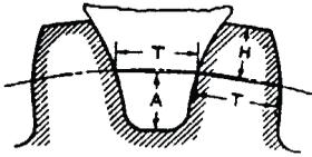
$T$  = chordal thickness of gear tooth and cutter tooth at pitch line;
