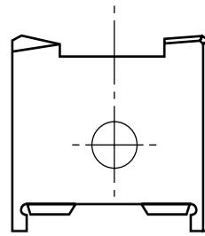
Fig. 2c. Core drilling blade
