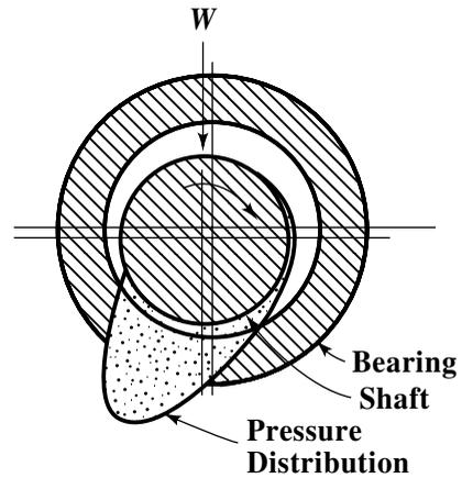
Fig. 2. Typical pressure profile of journal bearing.
