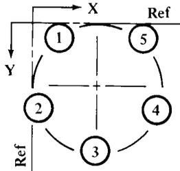
The diagram shows a type “B” circle for a 5-hole circle. Coordinates *x*, *y* are given in the table for hole circles of from 3 to 28 holes. Dimensions are for holes numbered in a counterclockwise direction (as shown). Dimensions given are based upon a hole circle of unit diameter. For a hole circle of, say, 3-inch or 3-centimeter diameter, multiply table values by 3.
