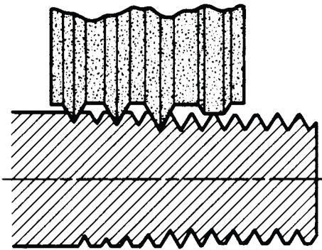
Fig. 1. Wheel with Edges for Roughing and Finishing
