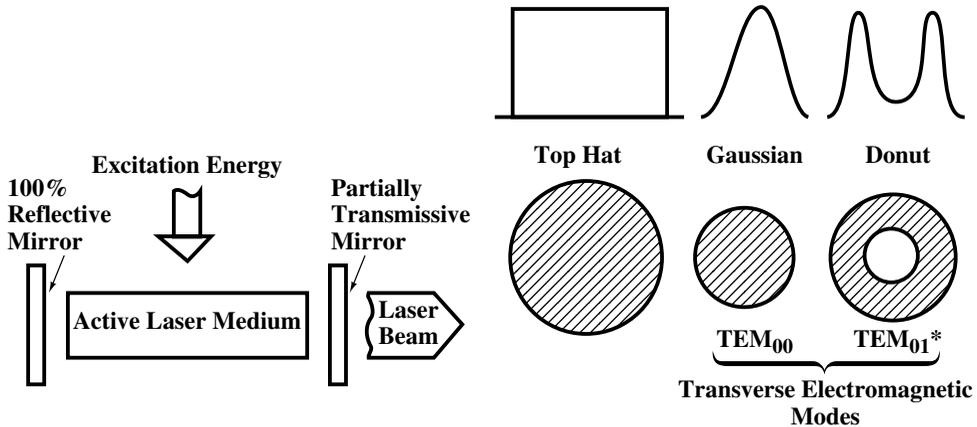
Fig. 1. Basic Components of a Laser
