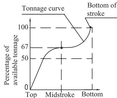
Fig. 71. Available Tonnage Curve for a Mechanical Press
