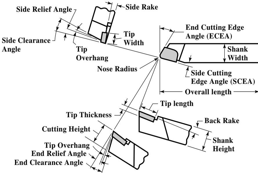
Fig. 2. A typical single-point carbide tipped cutting tool.
