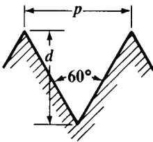
Owing to the difficulties connected with the V-thread, the tap manufacturers agreed in 1909 to discontinue the making of sharp V-thread taps, except when ordered. One advantage of the V-thread is that the same cutting tool may be used for all pitches, whereas, with the American Standard form, the width of the point or the flat varies according to the pitch.
