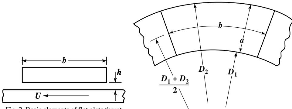
Fig. 2. Basic elements of flat plate thrust bearing.\*
