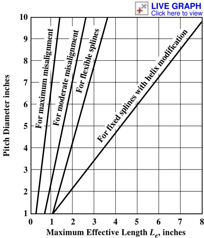
Fig. 4. Maximum Effective Length for Fixed and Flexible Splines = wear life factor from Table 10;  $L_e$  = maximum effective length from Fig. 4, to be used in stress formulas even though the actual length may be greater;  $T$  = transmitted torque, pound-inches. For fixed splines without helix modification, the effective length  $L_e$  should never exceed  $5000 D^{3.5} \div T$ .
