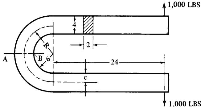
The cross-sectional area =  $2 \times 4 = 8$  square inches; the bending moment at section *AB* is  $1000(24 + 6 + 2) = 32,000$  inch pounds; the distance from the center of gravity of the section at *AB* to point *B* is  $c = 2$  inches; and using the formula on page 235, the moment of inertia of the section is  $2 \times (4)^3 \div 12 = 10.667$  inches<sup>4</sup>.
