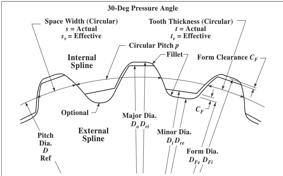
The fit shown is used in restricted areas (as with tubular parts with wall thickness too small to permit use of fillet roots, and to allow hobbing closer to shoulders, etc.) and for economy (when hobbing, shaping, etc., and using shorter broaches for the internal member).
