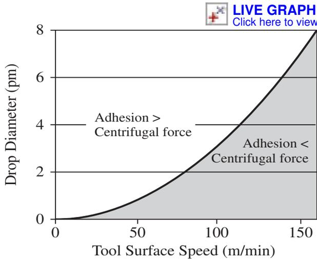
Fig. 25. Adhesion threshold of microdroplets on a rotating tool. CL2210EP lubricant, Ø1 mm uncoated carbide tool at different speeds. Note: 1pm = 1 picometer = 10<sup>-12</sup> meter.
