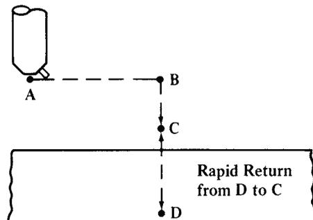
The G86 boring cycle is similar to the G85 cycle except that the tool is withdrawn at the rapid traverse rate.
