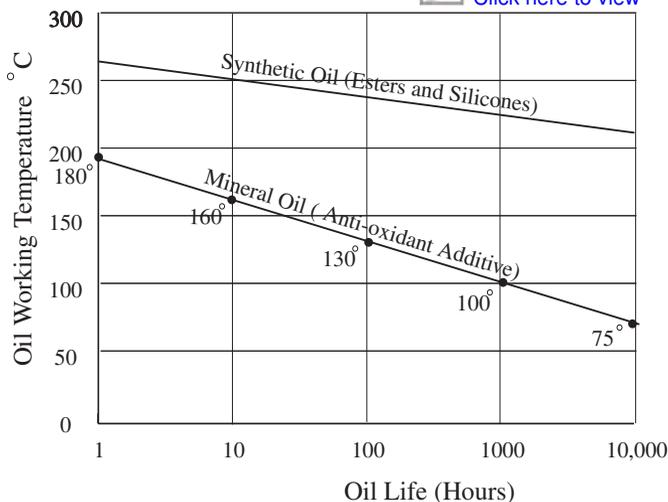
Fig. 8. Expected Oil Life at Varying Operating Temperatures.
