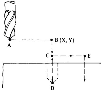
This G81 drilling cycle will move the drill point from position A to position B and then down to C at a rapid traverse rate; the drill point will next be fed from C to D at the programmed feed rate, then returned to C at the rapid traverse rate. If the cycle is to be repeated at a subsequent point, such as point E in the illustration, it is necessary Only to give the required X and Y coordinates. This repetition capability is typical of canned cycles.
