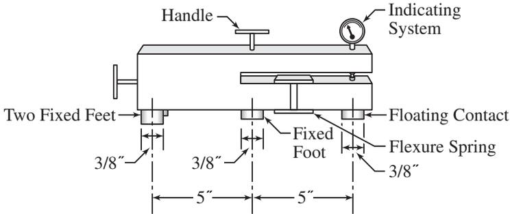
Fig. 2. Repeat Reading Gage from Federal Specification GGG-P-463c
