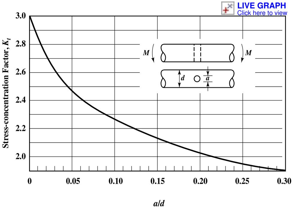
Fig. 10. Stress-concentration factor,  $K_t$ , for a shaft, with a transverse hole, in bending<sup>a</sup>
