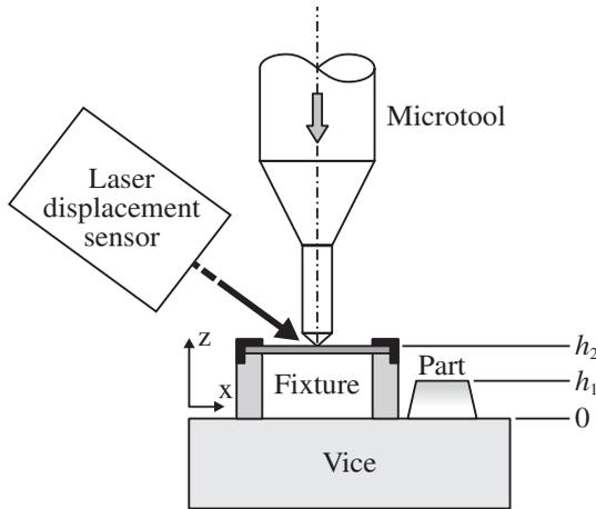
Fig. 9. Indirect vertical tool offset detection technique.
