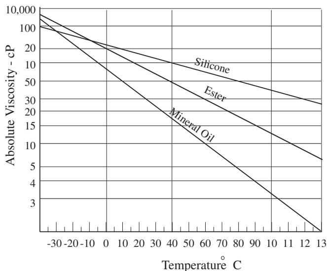
Fig. 7. Temperature Effect on Viscosity for Different Oils
