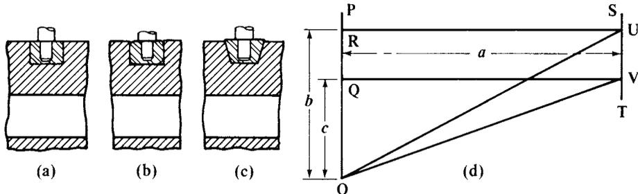
Fig. 23. Shape of Rolls for Cylinder Cams
