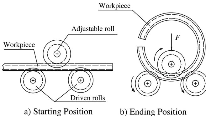
Fig. 69. Roll Bending: a) Starting Position; b) Finished
