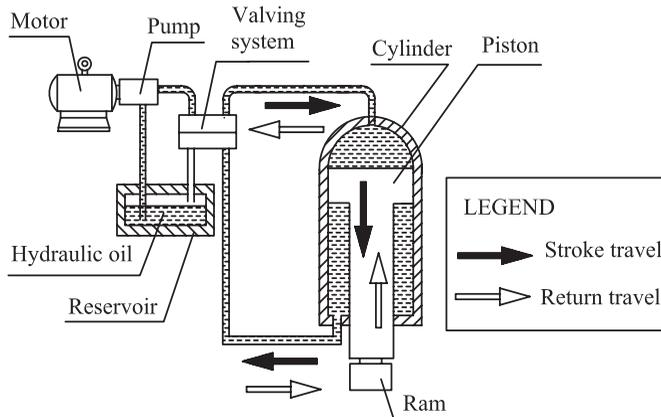
Fig. 73. Schematic Illustration of Hydraulic Press Drive System
