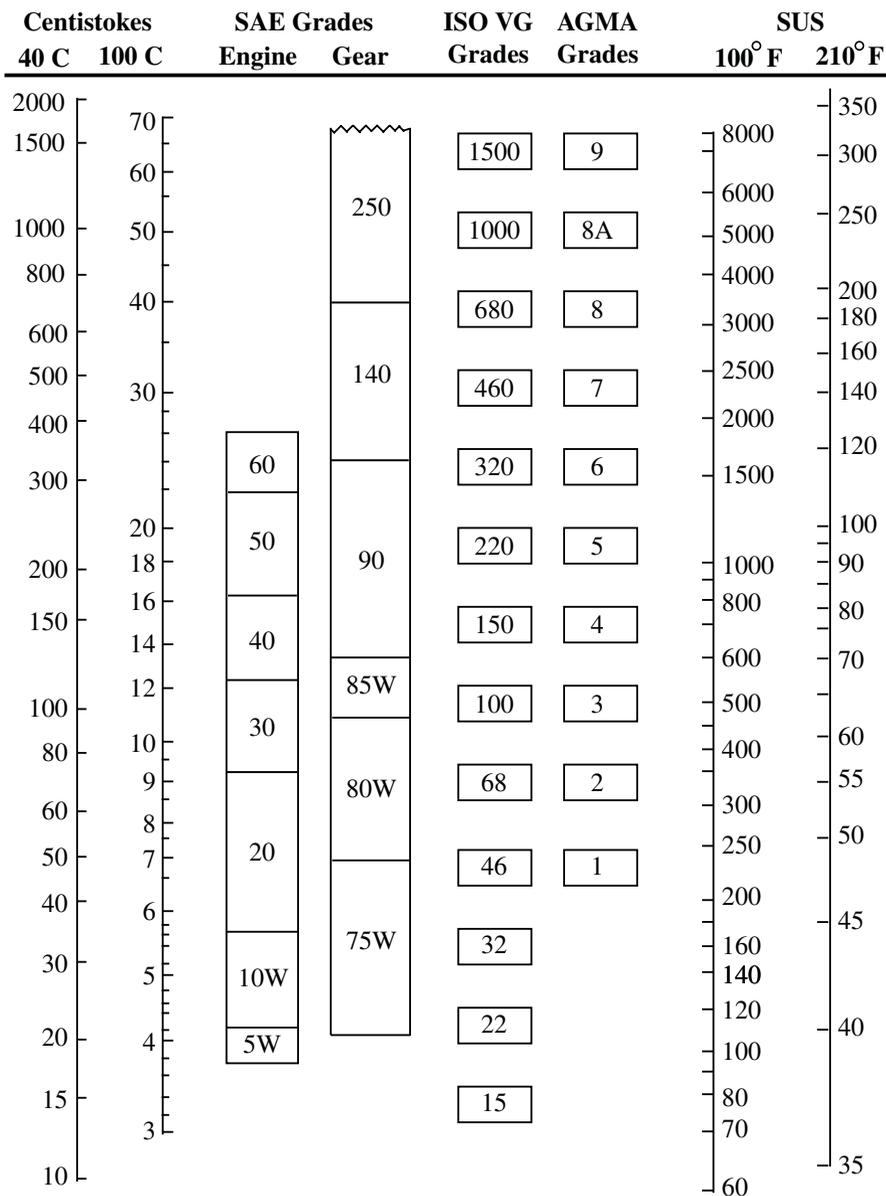
Viscosities based on 95VI single grades relate horizontally. SAE - Society of Automotive Engineers (Automotive lubricants)
