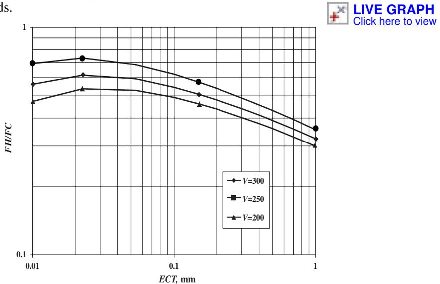
Fig. 10.  $F_H/F_C$  vs.  $ECT$ , cutting speed plotted
