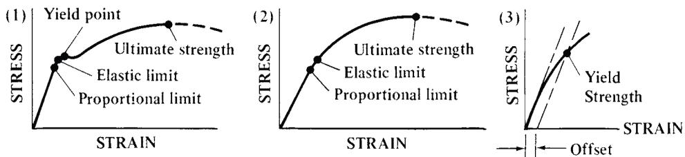
Fig. 1. Stress-strain curves
