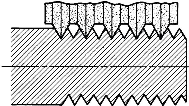
Fig. 3. Alternate-ribbed Wheel for Grinding the Finer Pitches
