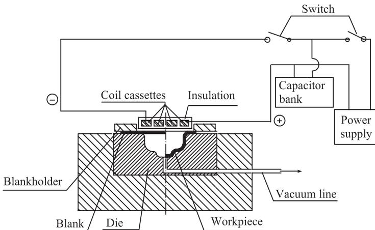
Fig. 31. Schematic Illustration of Electromagnetic Sheet Metal Forming
