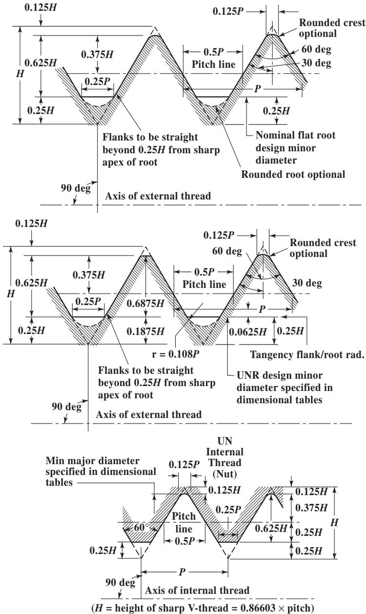
**Thread Series.**—Thread series are groups of diameter-pitch combinations distinguished from each other by the numbers of threads per inch applied to a specific diameter. The various diameter-pitch combinations of eleven standard series are shown in Table 2. The limits of size of threads in the eleven standard series together with certain selected combinations of diameter and pitch, as well as the symbols for designating the various threads, are given in Table 3. (Text continues on page 1844)
